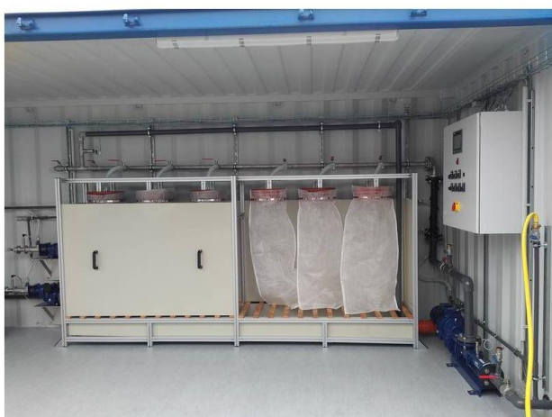
Figure 23: Example of the filtration bag technology proposed for the sludge treatment on site
