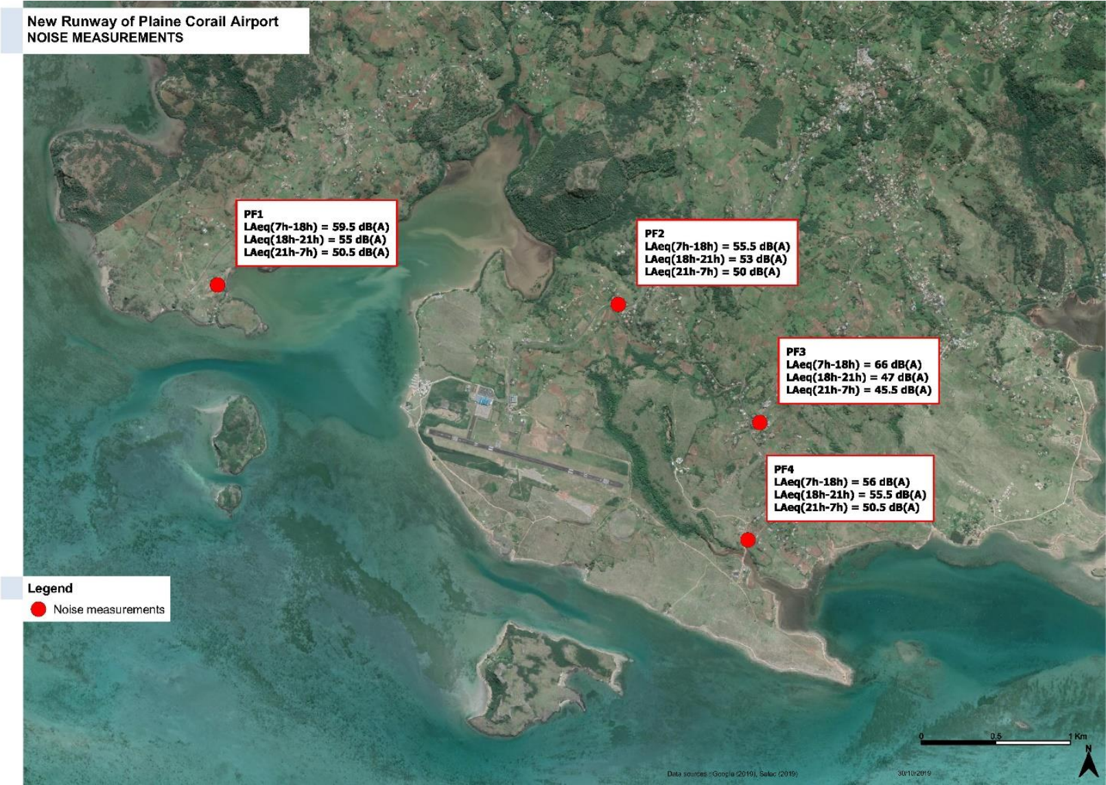
Figure 165 Noise measurements - location and results
