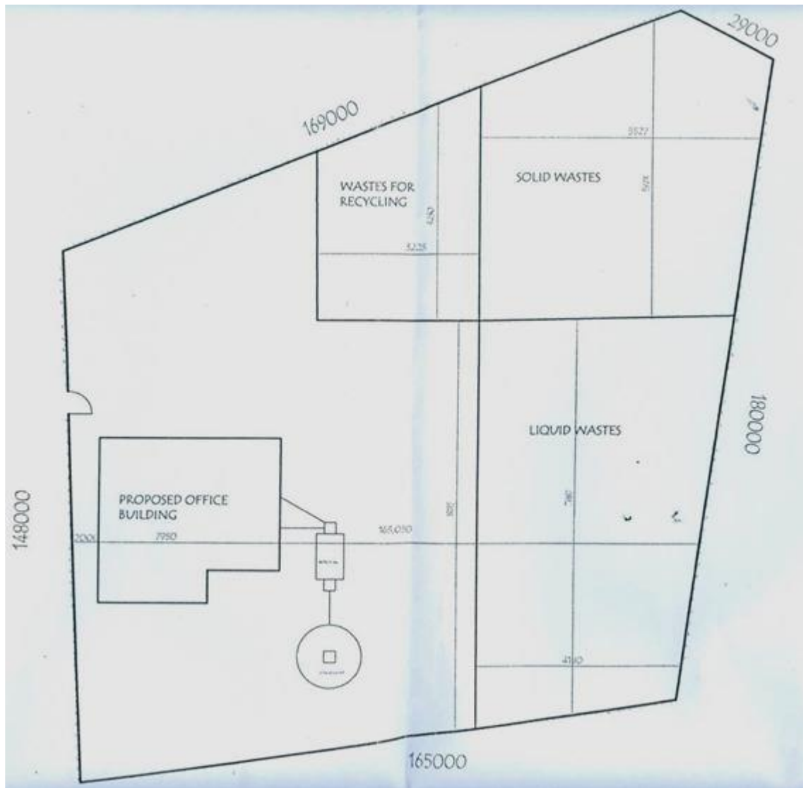
Figure 6 Proposed Layout Plan for Magu Solid Waste Disposal Site
