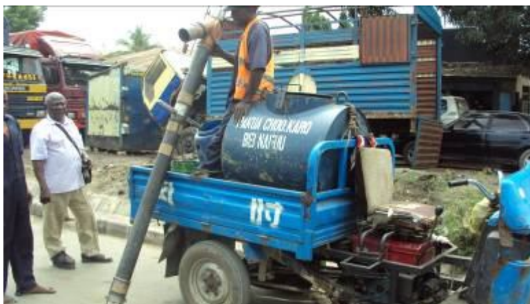
Figure 25: Example of the tricycle with a tank suitable for onsite disposal that may be adopted in tricky areas of Mabatini and Igogo.
