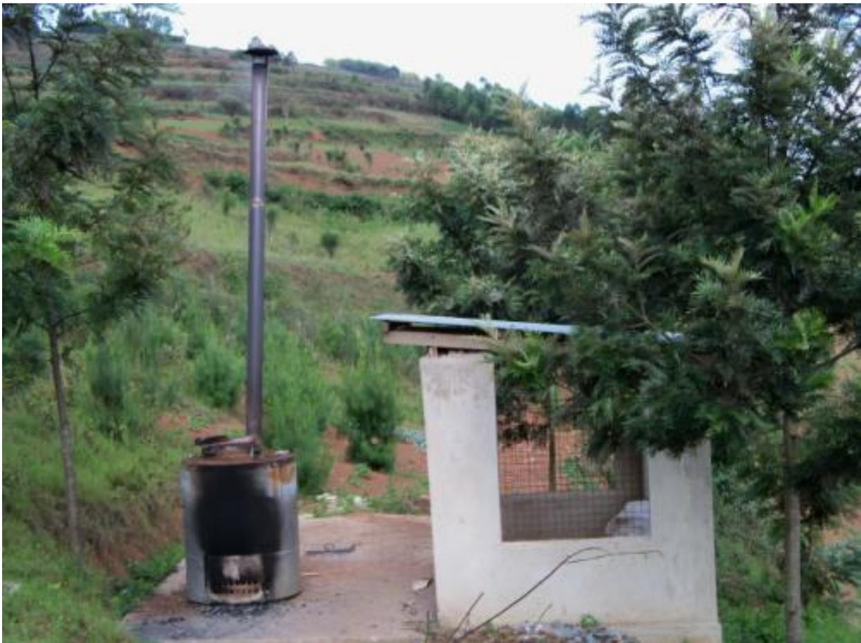
**Figure 13: MAK IV Incinerator**
