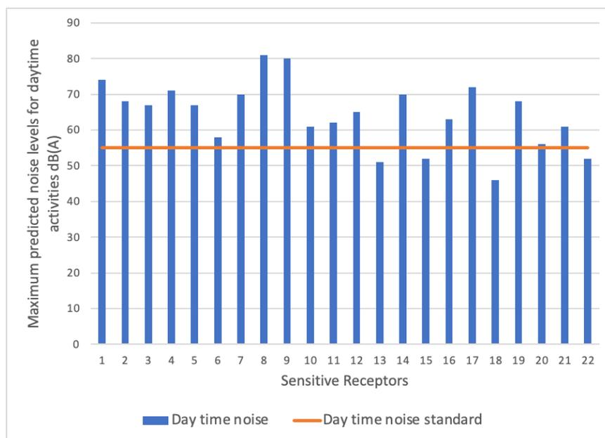
**Figure 68. Summary of predicted day time noise levels in the sensitive receptors compared to the Armenian Standard. The names of the sensitive receptors are given relative to the numbers in Table 39**
