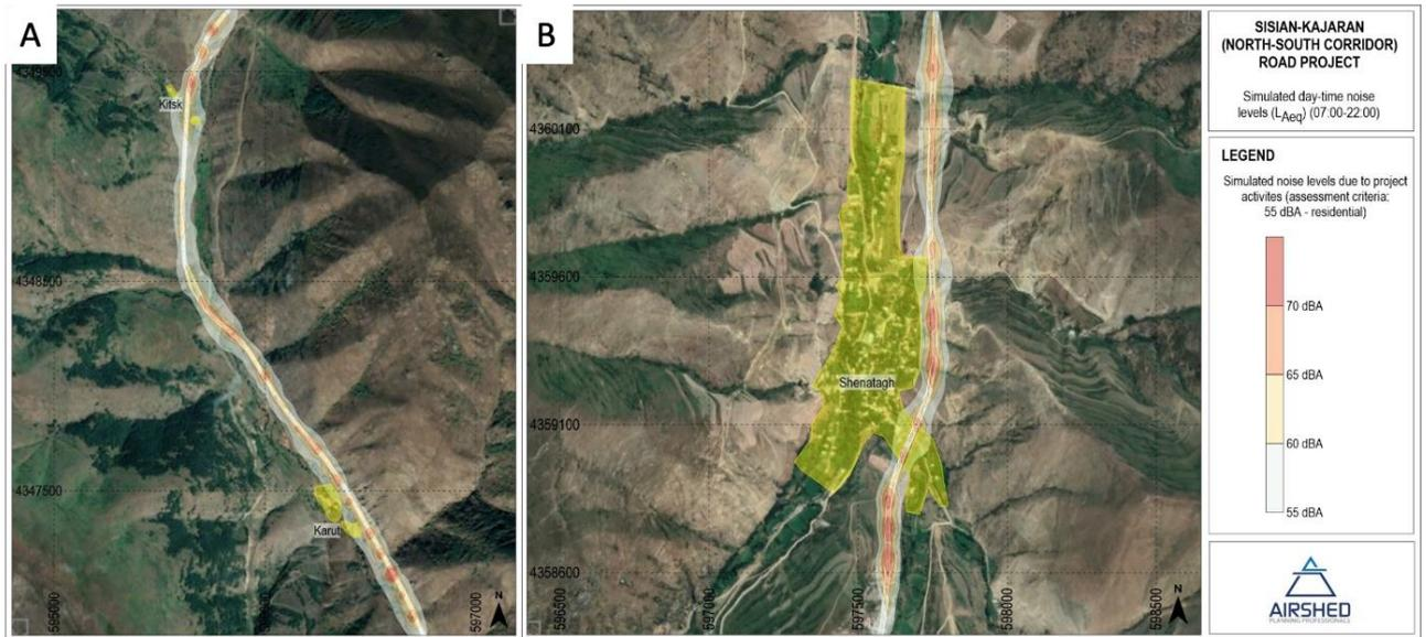
**Figure 76. Predicted day-time noise levels during operations of the roadway (2029) in study area 1. A=Site 2 and B=Site 3**
