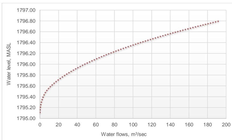
**Figure 34. Calculated water level increase during the spring flooding season under the planned bridge 016**
