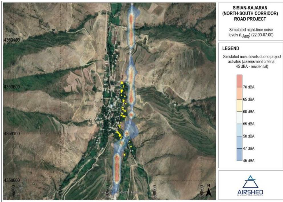
**Figure 90. Predicted noise levels for the section of road passing Shenatagh with a generic 8m wall as a noise barrier, relative to the Armenian nighttime standard of 45 dB(A)**
