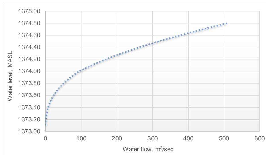
**Figure 33. Calculated water level increase during the spring flooding season under the planned bridge 005**
