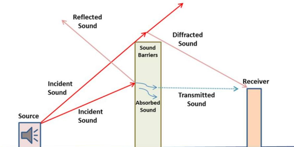
**Figure 84. The different physical mechanisms for noise barrier performance**
