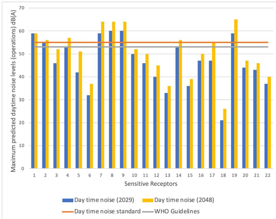
Figure 74. Predicted day-time noise levels during operations of the roadway (2029 and 2048) at sensitive receptors along the road alignment
