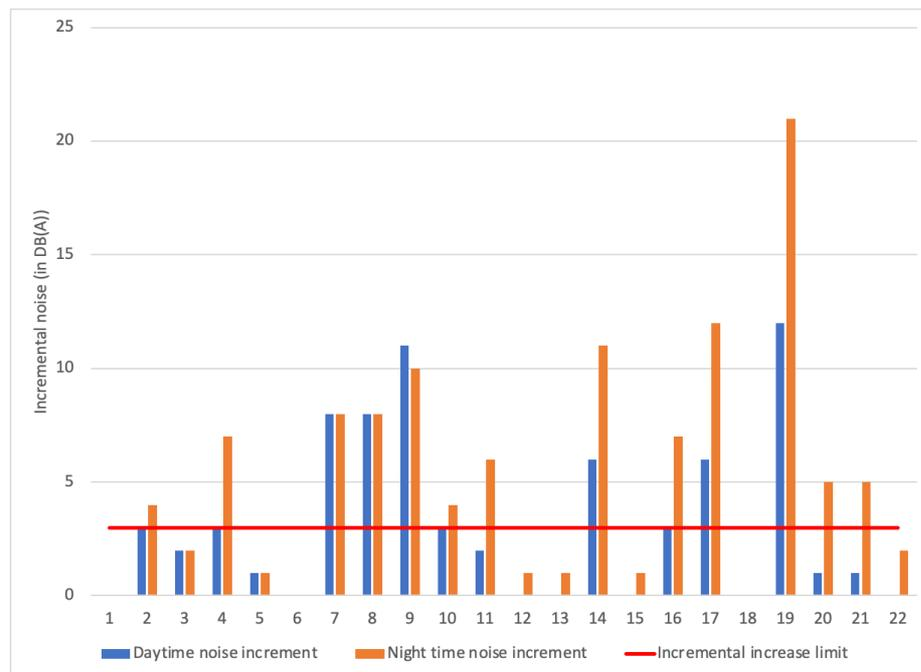
**Figure 83. Incremental noise as a result of the combination of the baseline noise and the modelled noise levels for the 2048 traffic fleet**
