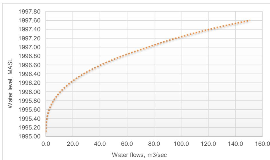
**Figure 36. Calculated water level increase during the spring flooding season under the planned bridge 018**
