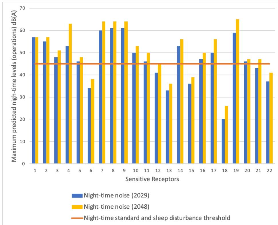
Figure 75. Predicted night-time noise levels during operations of the roadway (2029 and 2048) at sensitive receptors along the road alignment
