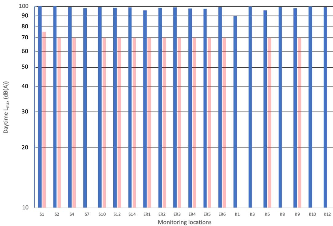
Figure 26. Daytime  $L_{max}$  noise measurements (blue bars) compared to the Armenian Standard (red bars)
