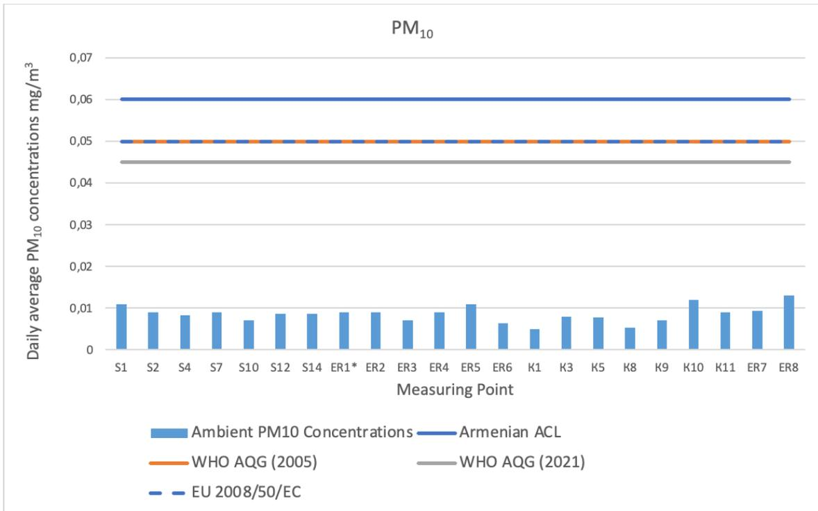
**Figure 16. Ambient daily average PM<sub>10</sub> concentrations as measured during the ESIA campaign, for various points along the road routing compared to the Armenian ACL and EU 2008/50/EC standards and WHO Air Quality Guidelines (2005 and 2021). The sampling points are summarised in Table 2**
