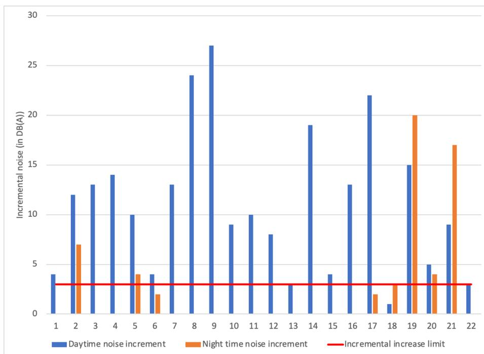
**Figure 71. Incremental noise as a result of the combination of the baseline noise and the modelled noise levels during construction**
