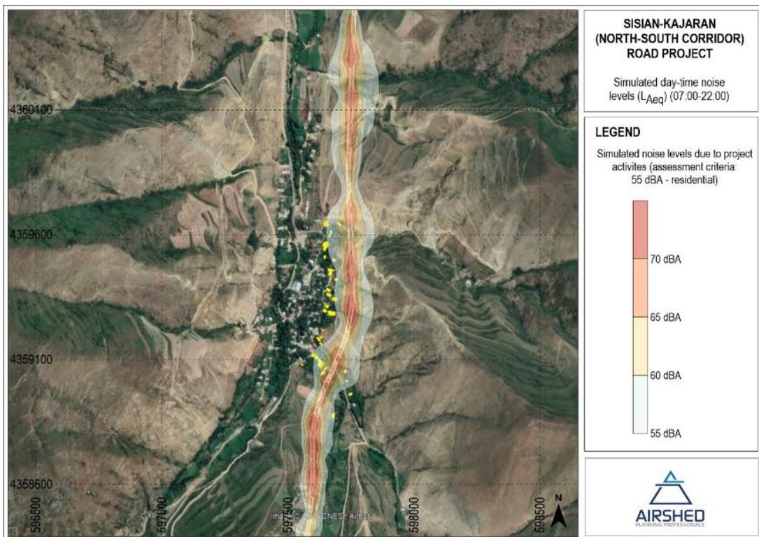
**Figure 87. Predicted unmitigated noise levels for the section of road passing Shenatagh in 2048 relative to the Armenian daytime standard of 55 dB(A)**
