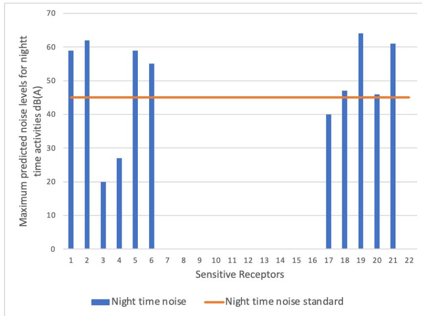
**Figure 69. Summary of predicted night time noise levels in the sensitive receptors compared to the Armenian Standard. The names of the sensitive receptors are given relative to the numbers in Table 39**
