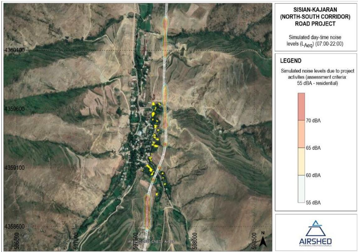
**Figure 88. Predicted noise levels for the section of road passing Shenatagh in 2048 with a generic 8m wall as a noise barrier, relative to the Armenian daytime standard of 55 dB(A)**
