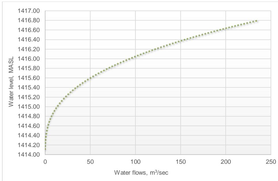
**Figure 35. Calculated water level increase during the spring flooding season under the planned bridge 021**
