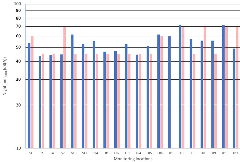
Figure 25. Night time  $L_{aeq}$  noise measurements (blue bars) compared to the Armenian Standard (red bars)
