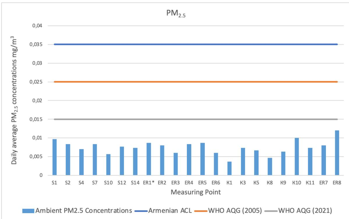
**Figure 15. Ambient daily average PM<sub>2.5</sub> concentrations as measured during the ESIA campaign, for various points along the road routing compared to the Armenian ACL and WHO Air Quality Guidelines (2005 and 2021). The sampling points are summarised in Table 2**
