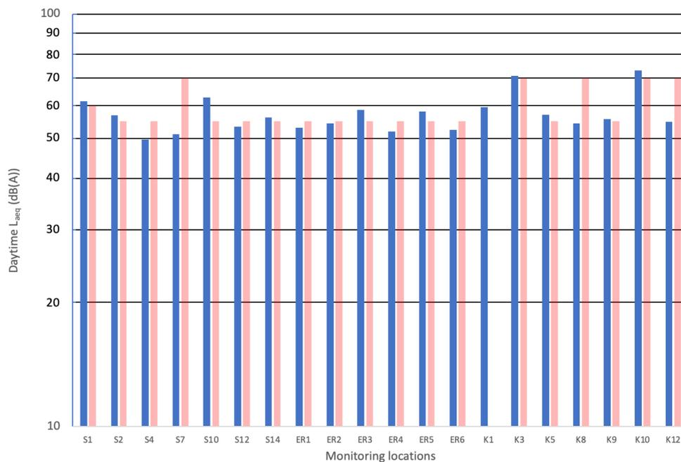
**Figure 24. Daytime  $L_{aeq}$  noise measurements (blue bars) compared to the Armenian Standard (red bars)**
