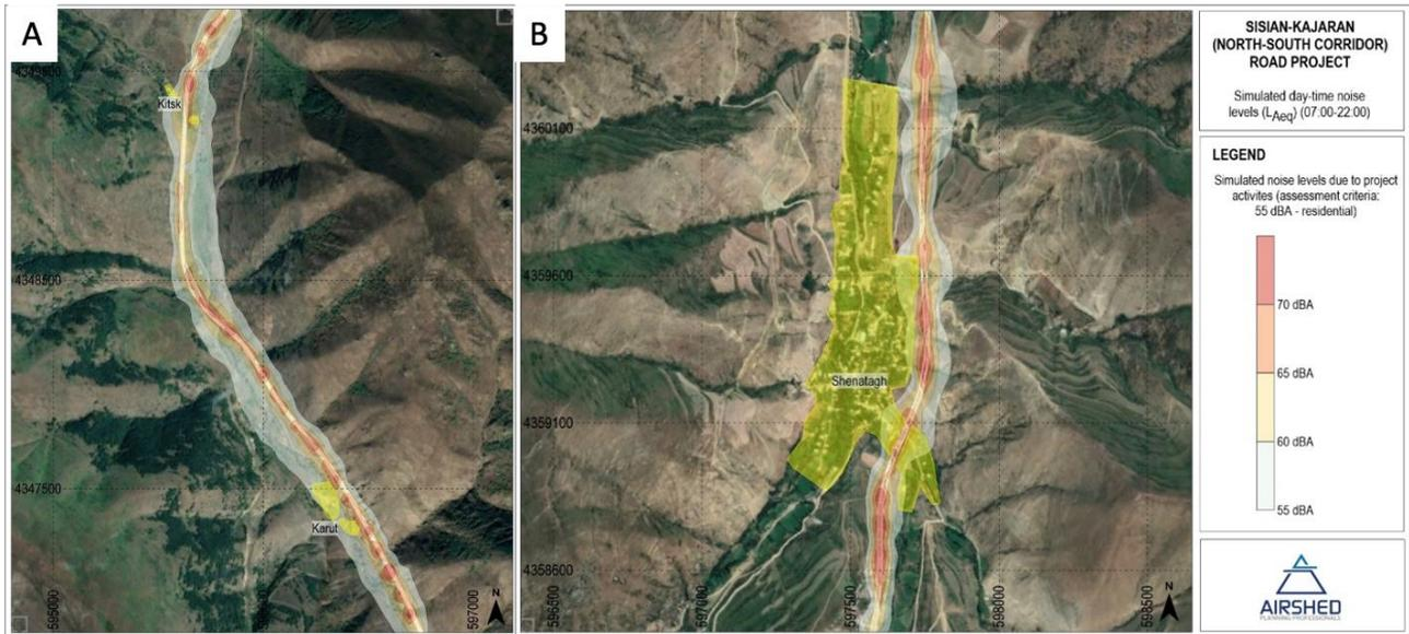
Figure 79. Predicted day-time noise levels during operations of the roadway (2048) in study area 1. A=Site 2 and B=Site 3
