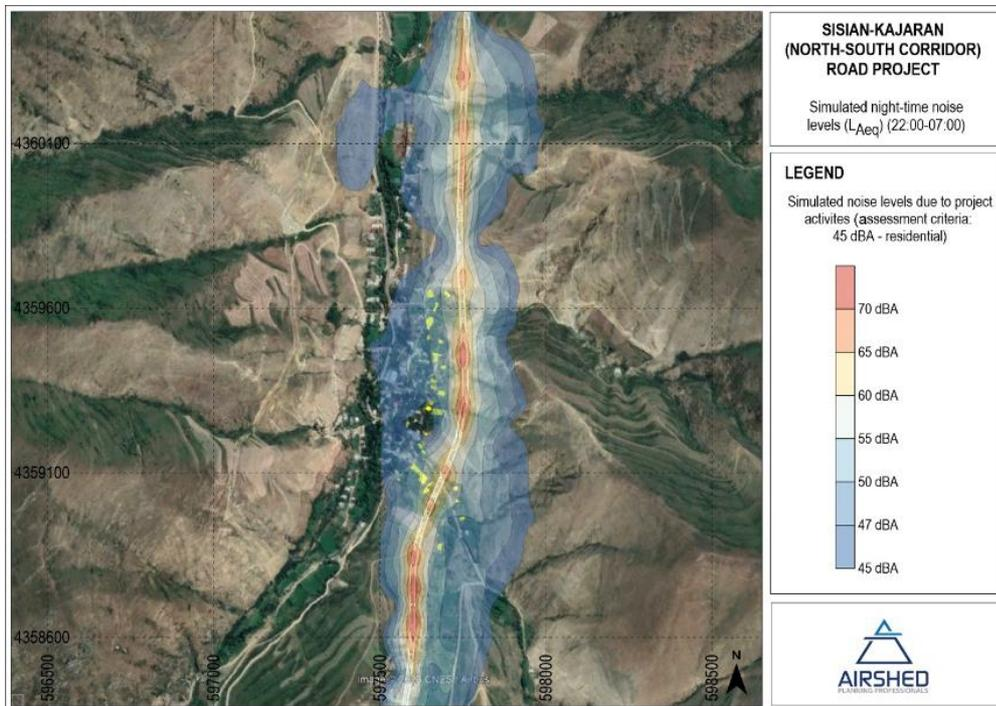
**Figure 89. Predicted unmitigated noise levels for the section of road passing Shenatagh relative to the Armenian night time standard of 45 dB(A)**
