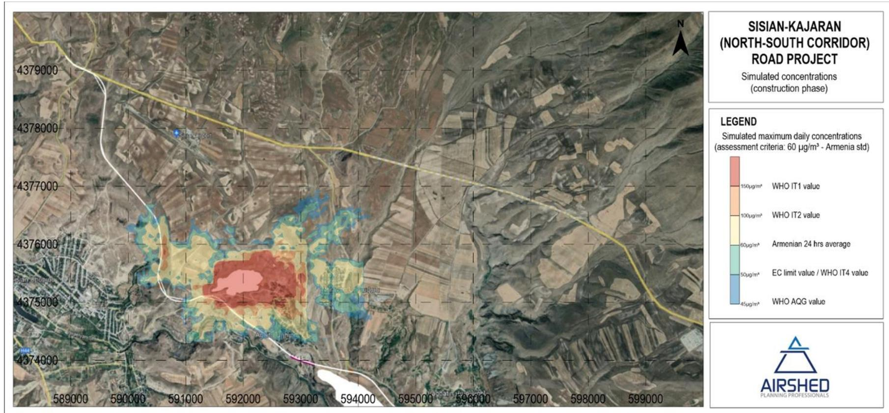
**Figure 57. Simulated highest daily average ambient PM<sub>10</sub> concentrations at Site 6 due to proposed project construction activities**
