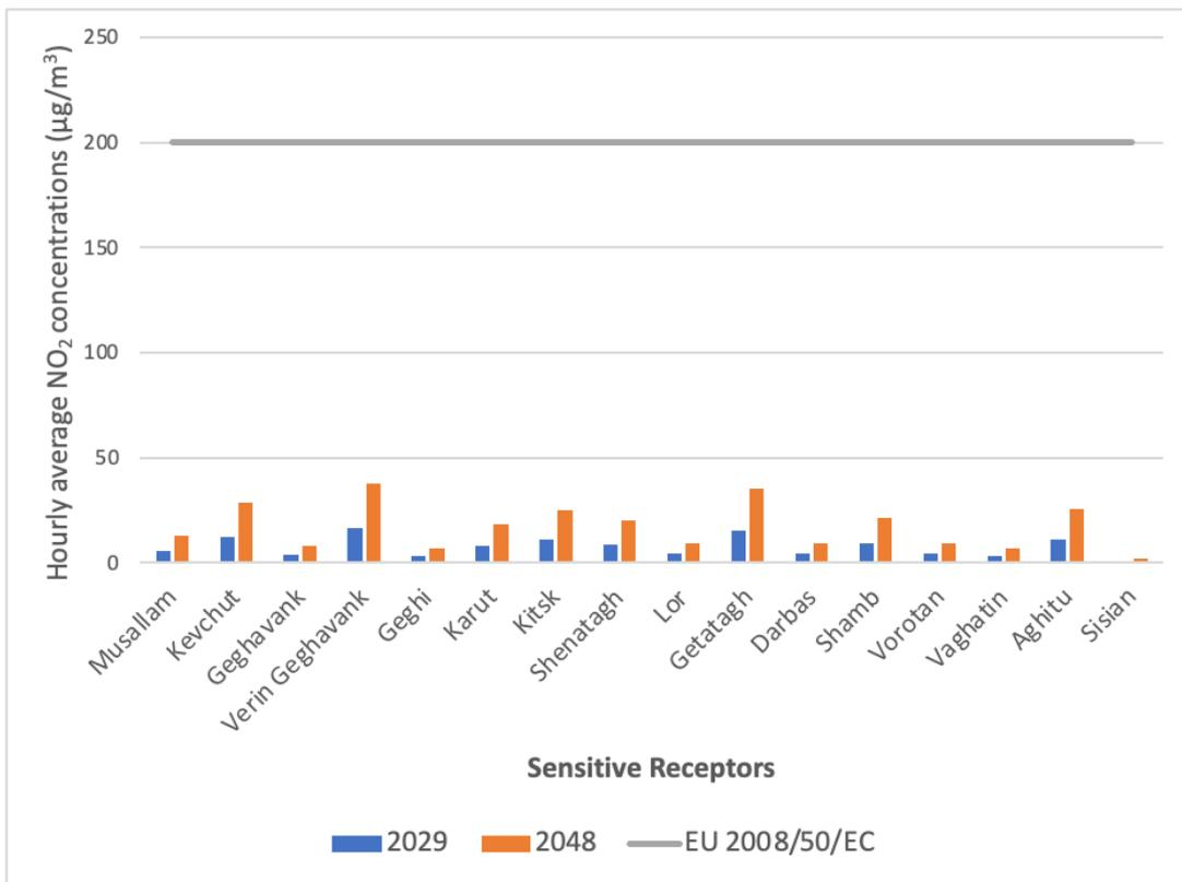
Figure 62. Predicted hourly average NO<sub>2</sub> concentrations at the various sensitive receptors along the proposed roadway for the 2029 and 2048 traffic fleet
