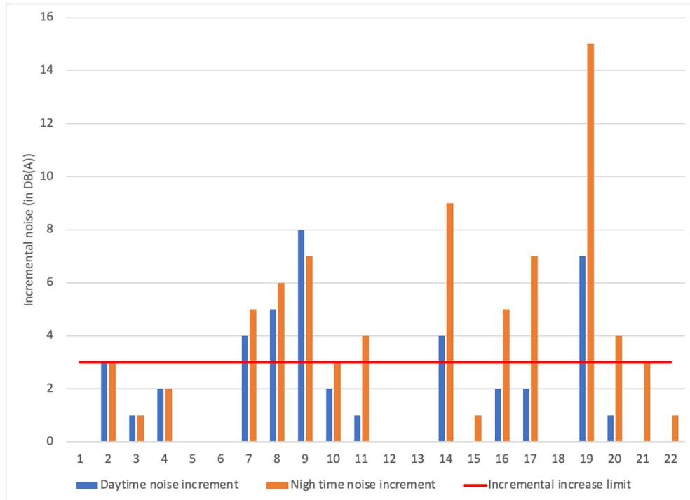
**Figure 82. Incremental noise as a result of the combination of the baseline noise and the modelled noise levels for the 2029 traffic fleet.**
