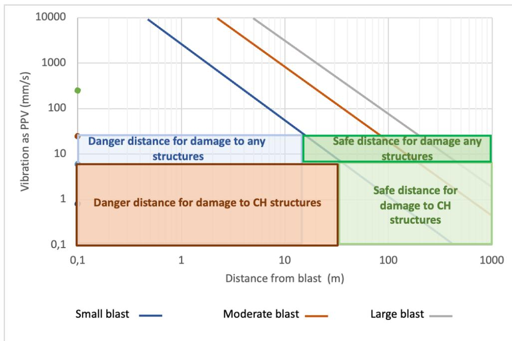
**Figure 73. Conceptual interpretation of Figure 72 to assist in understanding the implication of the scatter plot for heritage and other structures**
