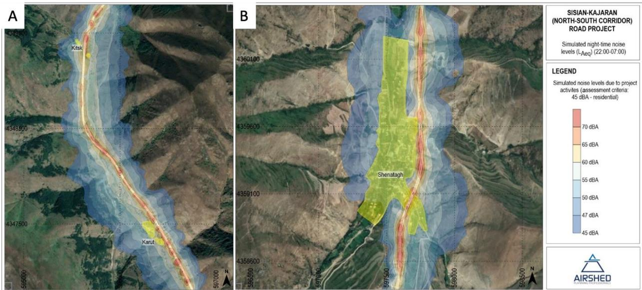
Figure 80. Predicted night-time noise levels during operations of the roadway (2048) in study area 1. A=Site 2 and B=Site 3
