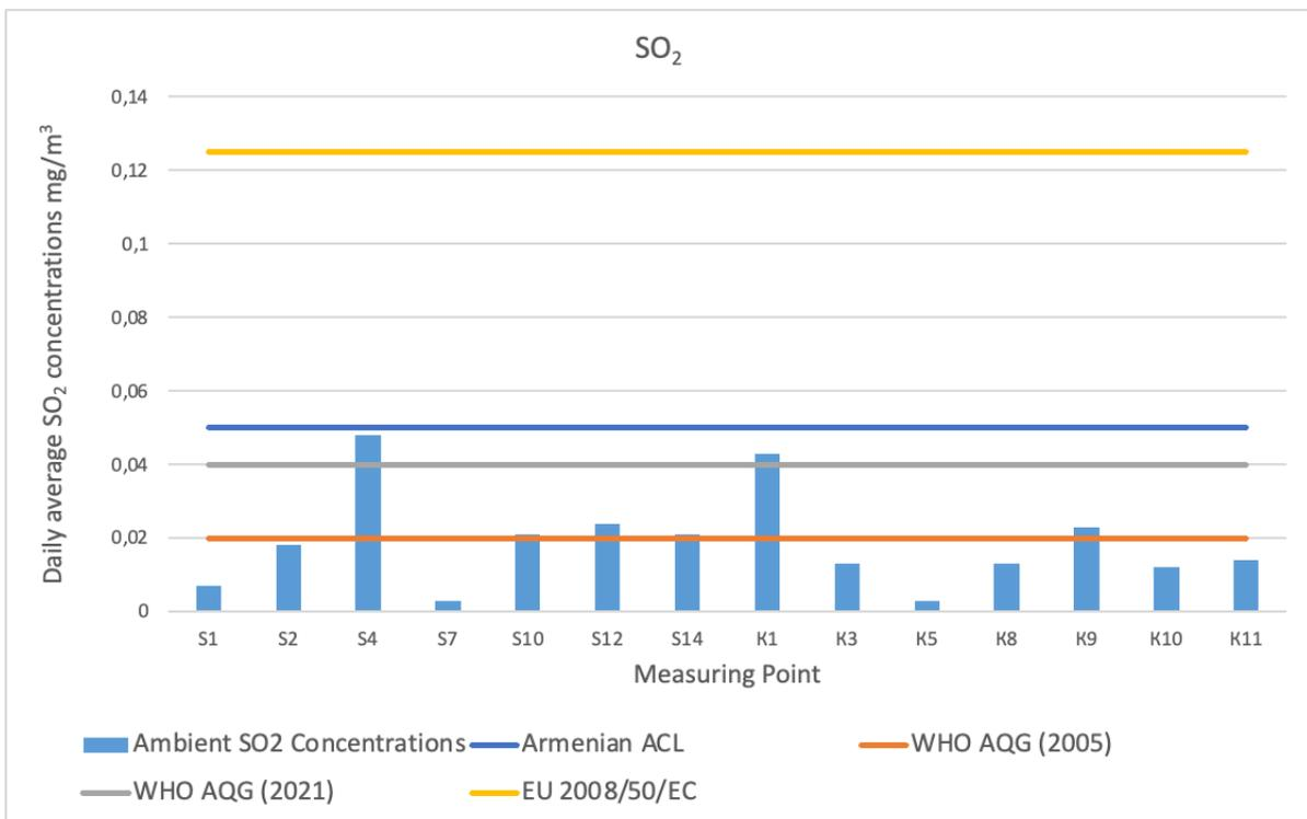
**Figure 17. Ambient daily average SO<sub>2</sub> concentrations as measured during the ESIA campaign, for various points along the road routing compared to the Armenian ACL and EU 2008/50/EC standards and WHO Air Quality Guidelines (2005 and 2021). The sampling points are summarised in Table 2**
