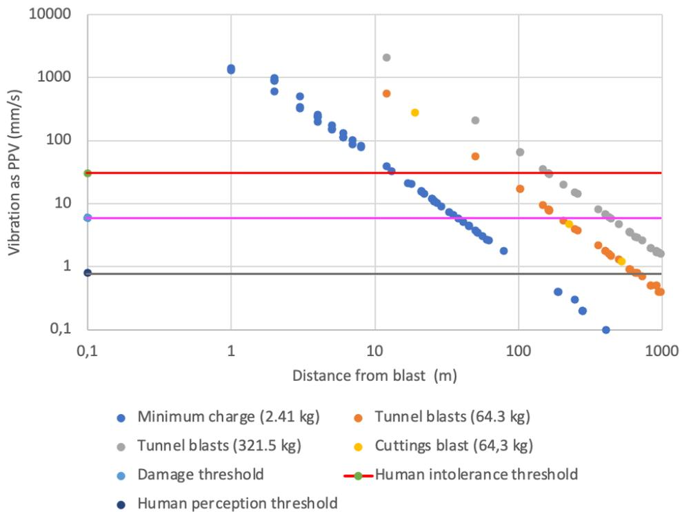
**Figure 72. Scatterplot of the vibration that would be received by the heritage structures identified along the roadway for different blast charges. Note that both axes are plotted logarithmically**
