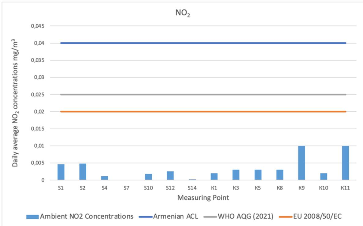
**Figure 14. Ambient daily average NO<sub>2</sub> concentrations as measured during the ESIA campaign, for various points along the road routing compared to the Armenian ACL, and WHO Air Quality Guidelines (2021). Note that there is no hourly limit for NO<sub>2</sub> in the 2005 guidelines. The sampling points are summarised in Table 2**
