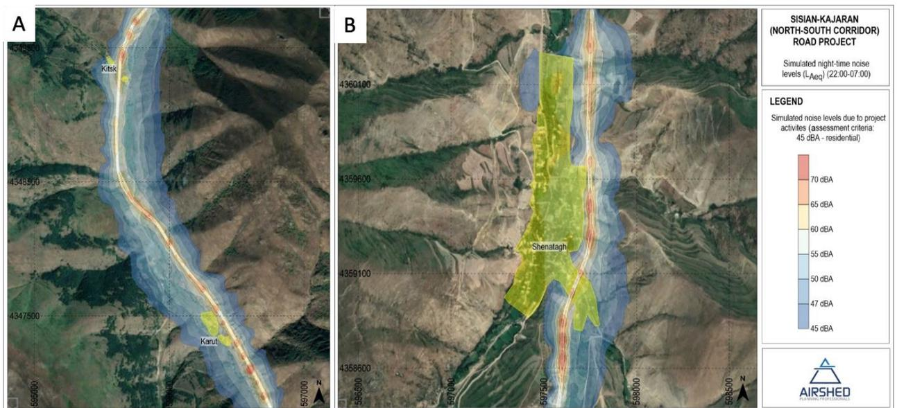
**Figure 77. Predicted night-time noise levels during operations of the roadway (2029) in study area 1. A=Site 2 and B=Site 3**
