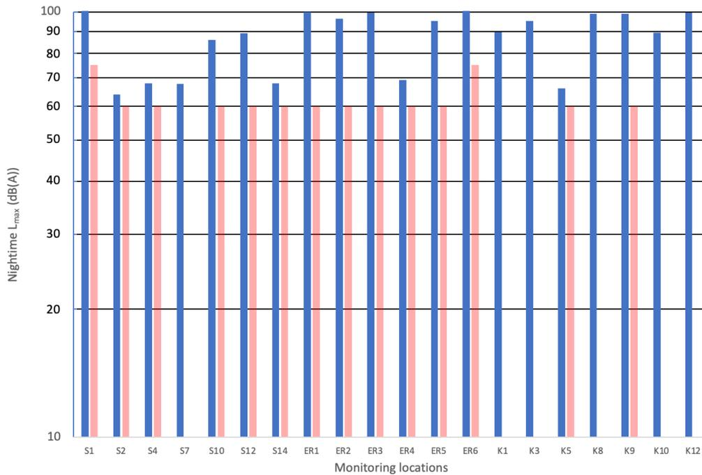
**Figure 27. Night time  $L_{max}$  noise measurements (blue bars) compared to the Armenian Standard (red bars)**
