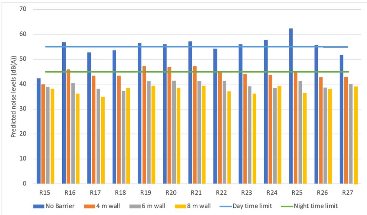
**Figure 91. The effect of noise barriers of differing heights in attenuating noise from the 2048 operational roadway for 27 sensitive receptors identified in Shenatagh, relative to the Armenian noise limits**
