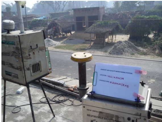
Photo-1: Ambient Air Quality Sampling at Kanja Gola
