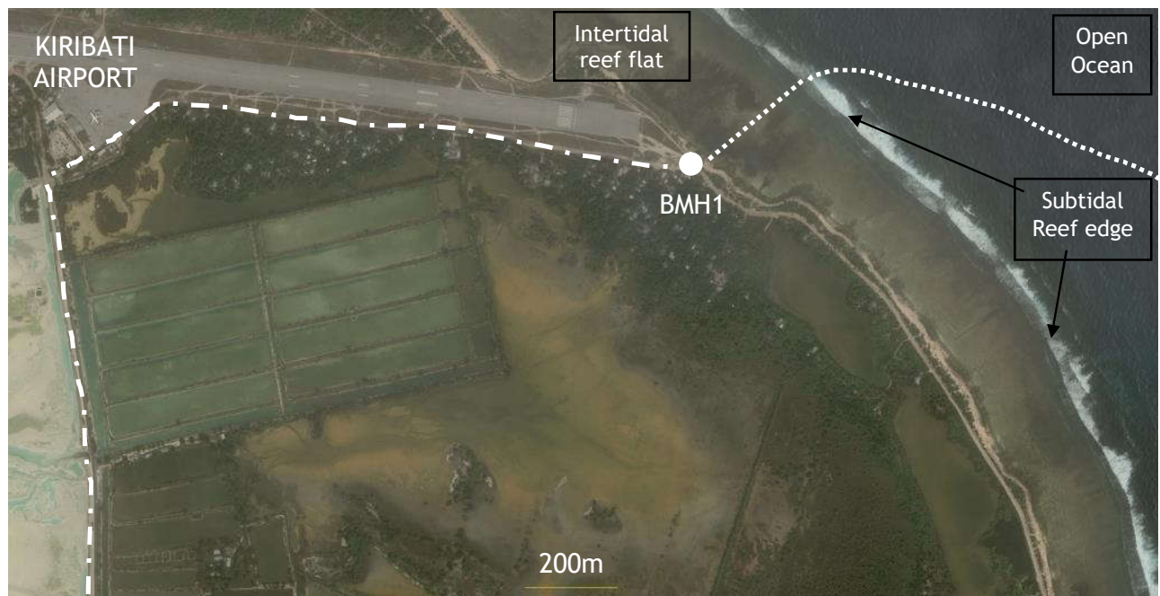
Figure 4f: Potential submarine and terrestrial cable alignments for BMH1 (white dashed lines) in Kiribati.
