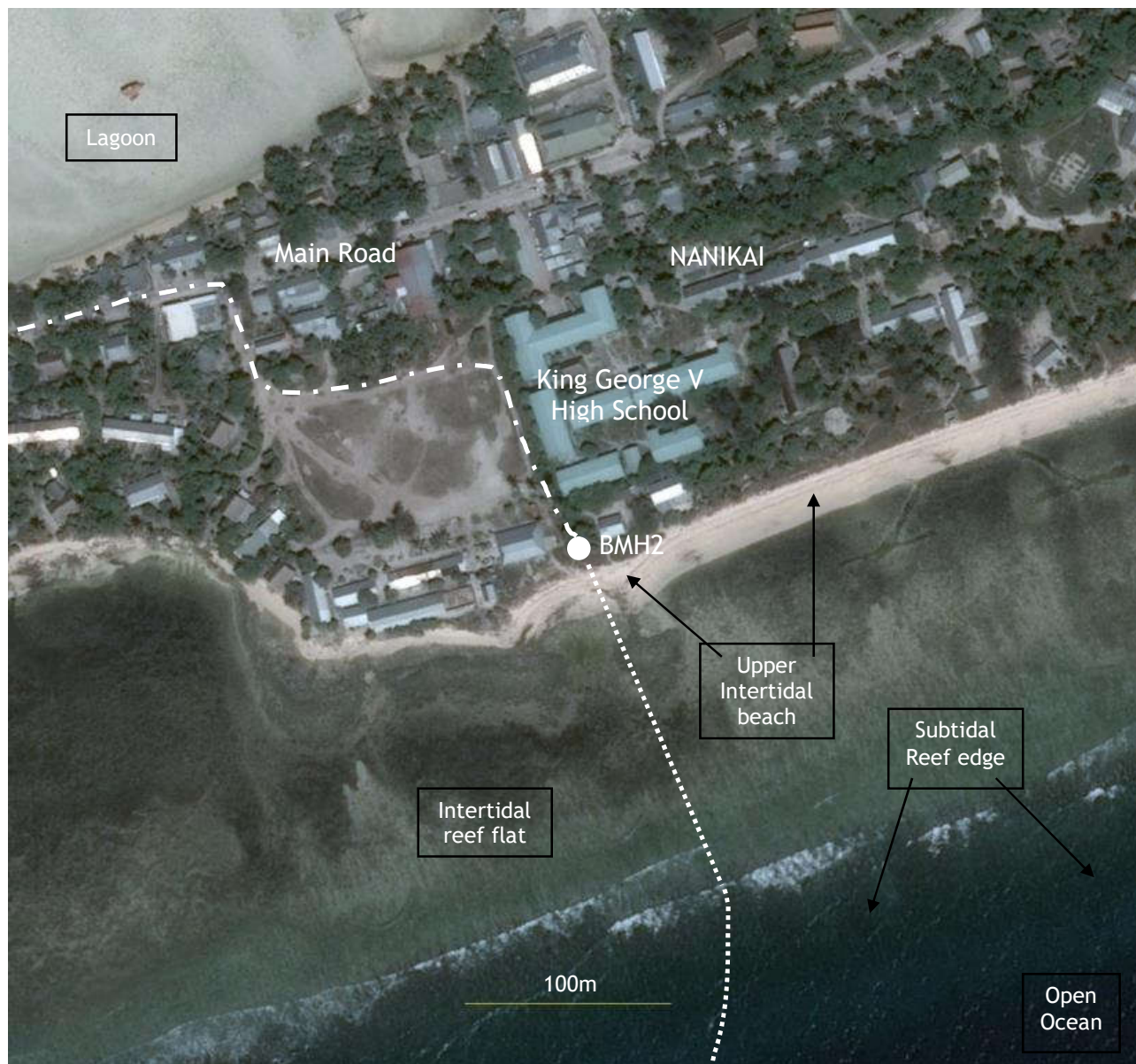
Figure 4g: Potential submarine and terrestrial cable alignments for BMH2 (white dashed lines) in Kiribati.
