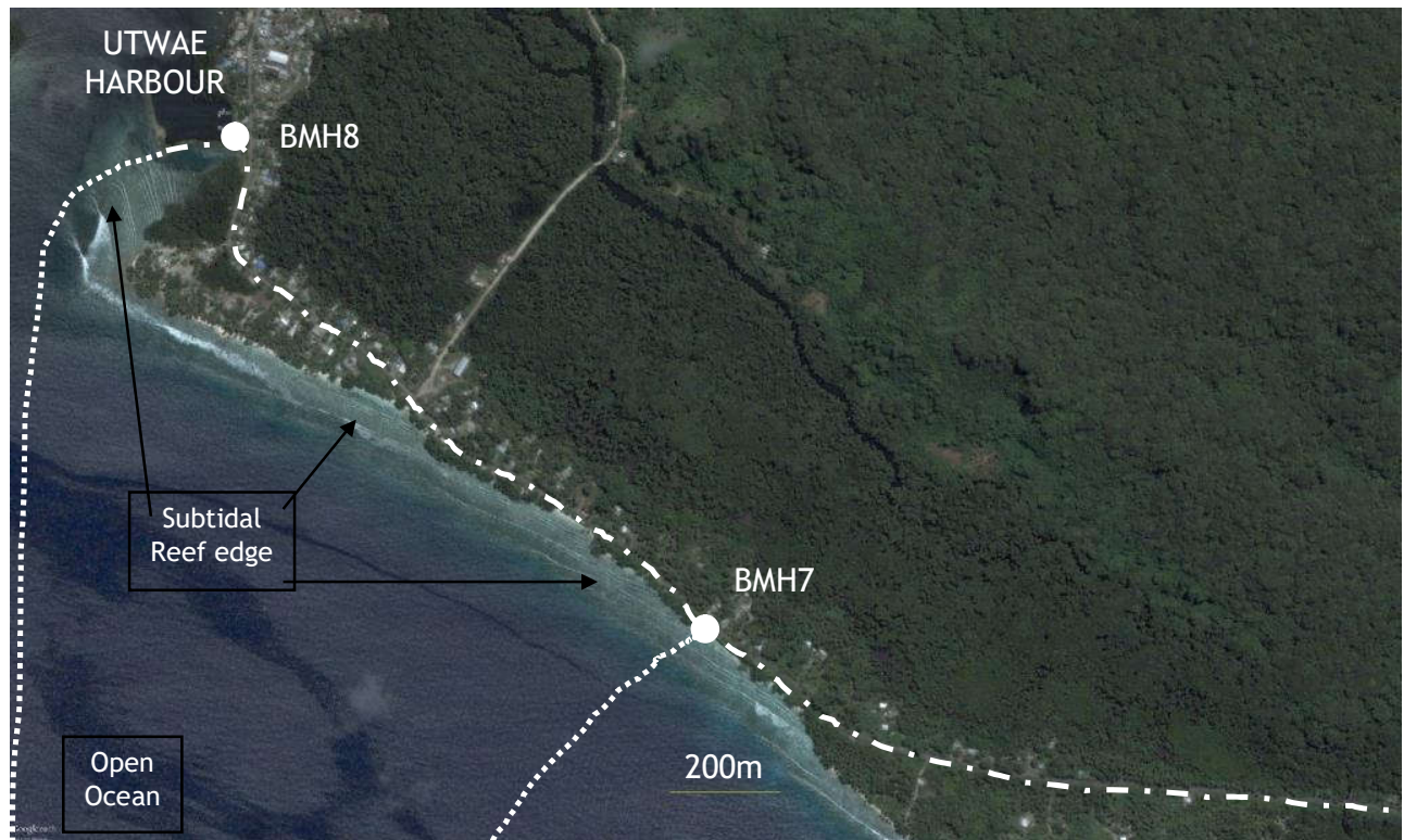
Figure 4e: Potential submarine and terrestrial cable alignments for BMH7 & 8 (white dashed lines) in Kosrae.
