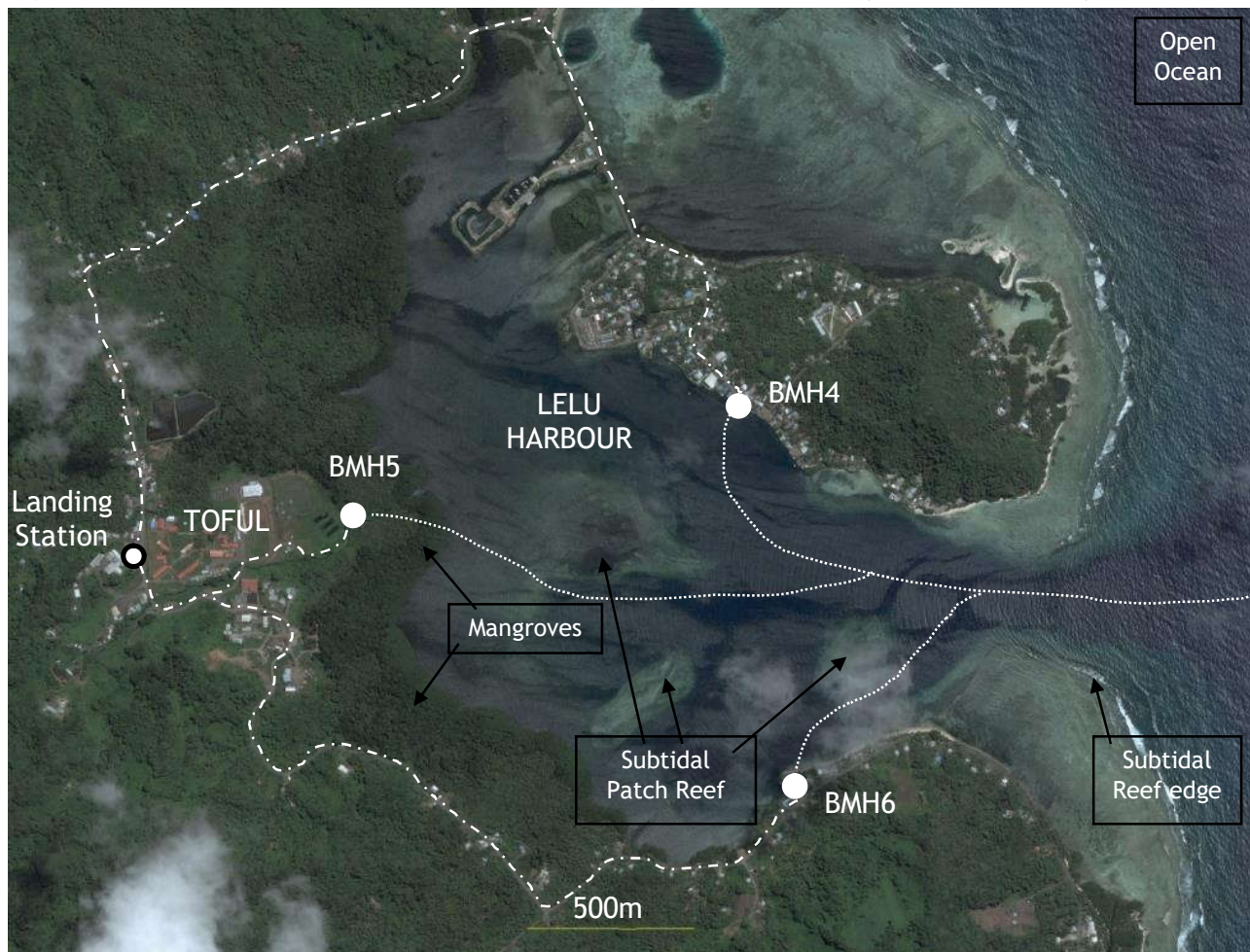
Figure 4c: Potential submarine and terrestrial cable alignments for BMH4, 5 & 6 (white dashed lines) in Kosrae.
