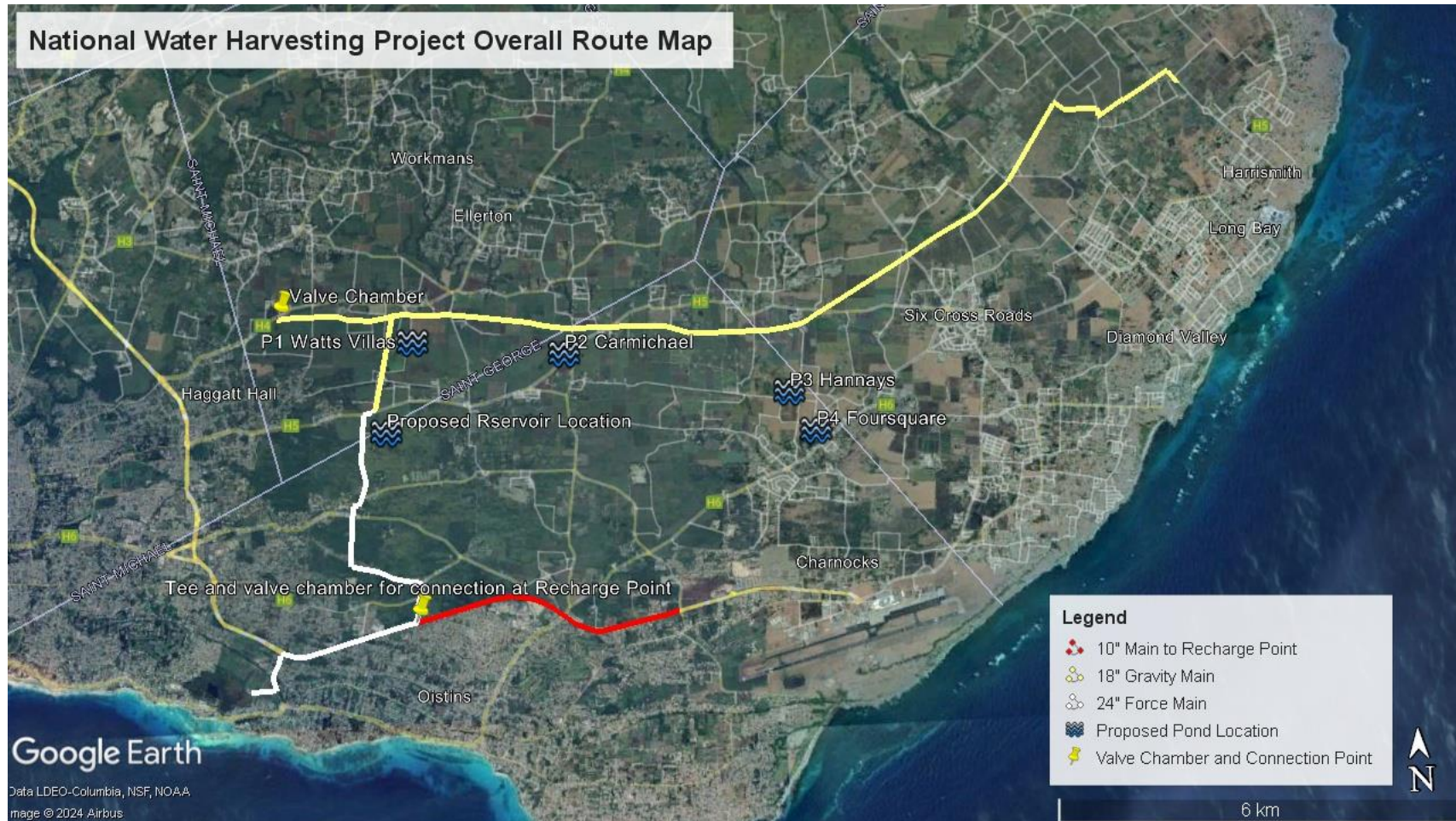
Figure 2-3: Route Map of Proposed Pipelines to be Installed and Proposed Catchment Ponds as Components of the Project
