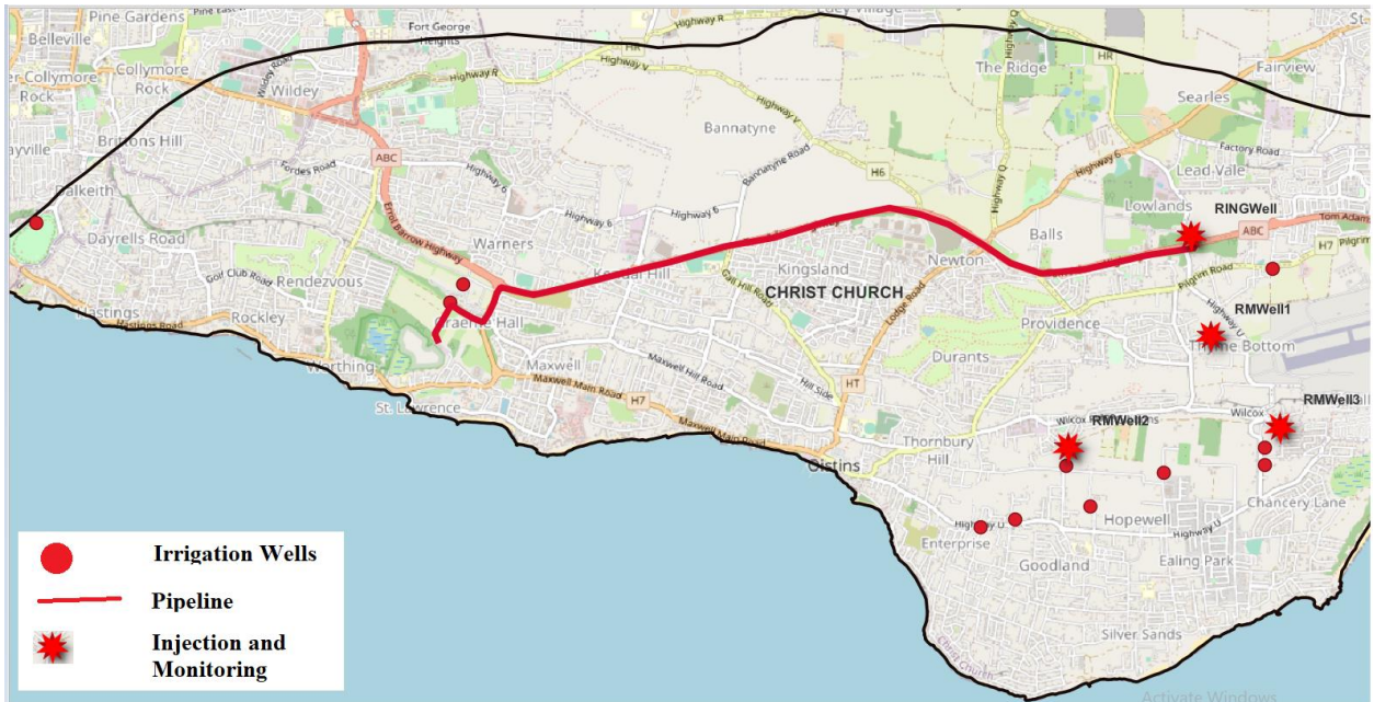
Pipeline from the South Coast Sewage Treatment Plant to Recharge Aquifer in Christ Church
