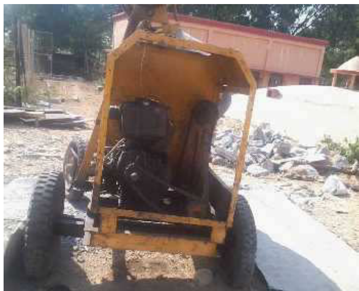
Concrete mixer without cover for the chains
