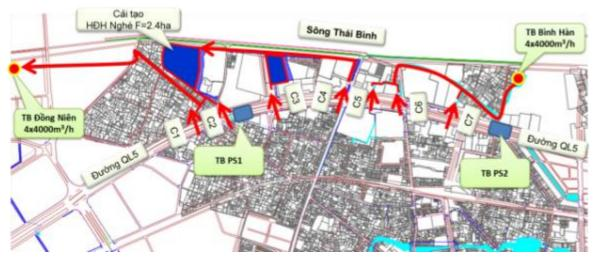
Figure 1.6: Rehabilitation Options for the Catchment Area in the North of the Railway
