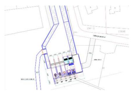
Figure 1.5: Typical Layout of Lo Cuong pumping station
