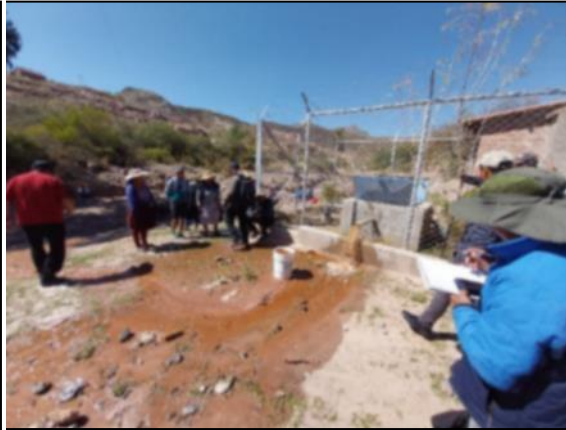
Aforo Pajchapata Lux (Q=5.40 lts/seg)
