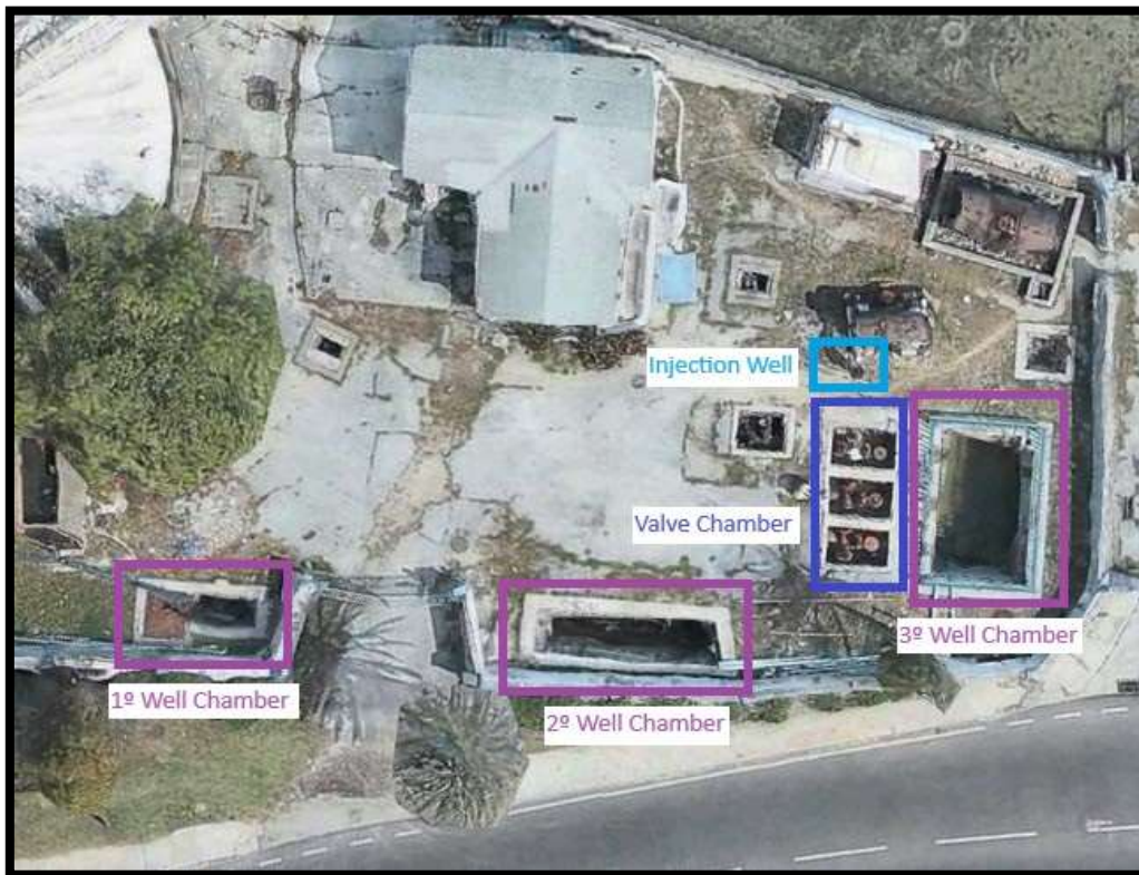
Figure 33. Malcom Lift Station Layout. Source: PlanEHS, 2024.
