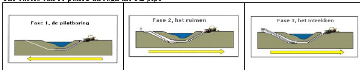
Figure 6: Phases of the HDD process
