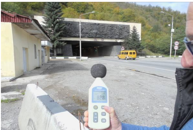
Figure 5.1. Noise measuring at the East portal of Rikoti tunnel
