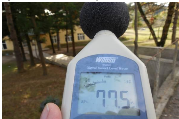
Figure 5.2. Noise measuring on the existing road, near a public school in Khevi
