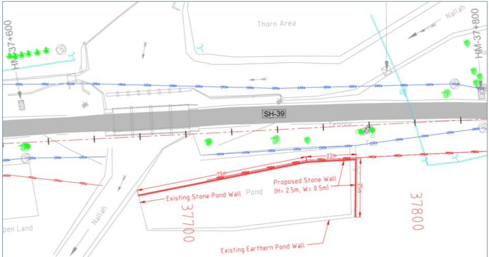
Drawing No. 3: Enhancement Measure for Pond at Chainage 37/600
