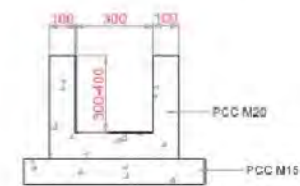
DETAIL "A" CROSS SECTION OF COLLECTION DRAIN Scale 1 : 10
