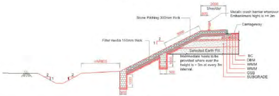
SECTION "B-B" SCALE 1 : 50
