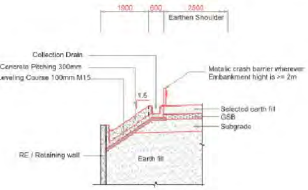
EMBANKMENT WITH CHUTE DRAIN AND COLLECTION PIT ARRANGEMENT @ UNDERPASS LOCATIONS
