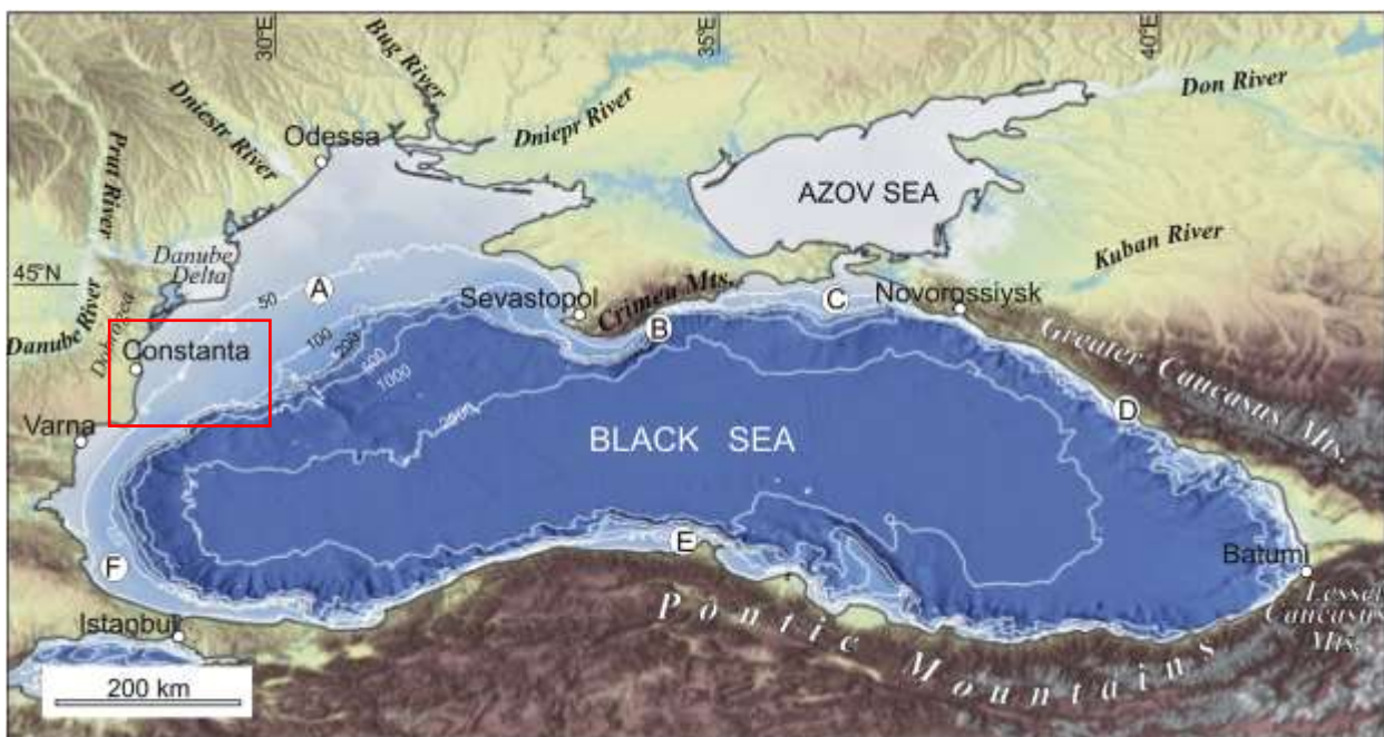
Figure 6-87 – Black Sea morphology and bathymetry. The Aol is highlighted in red. A) Northwestern Shelf. B) Crimea Shelf. C) Kerch-Taman Shelf. D) Caucasian Shelf. E) Anatolian Shelf. F) Bulgarian-Western Turkish Shelf. (Source: Jipa & Panin, 2020).
