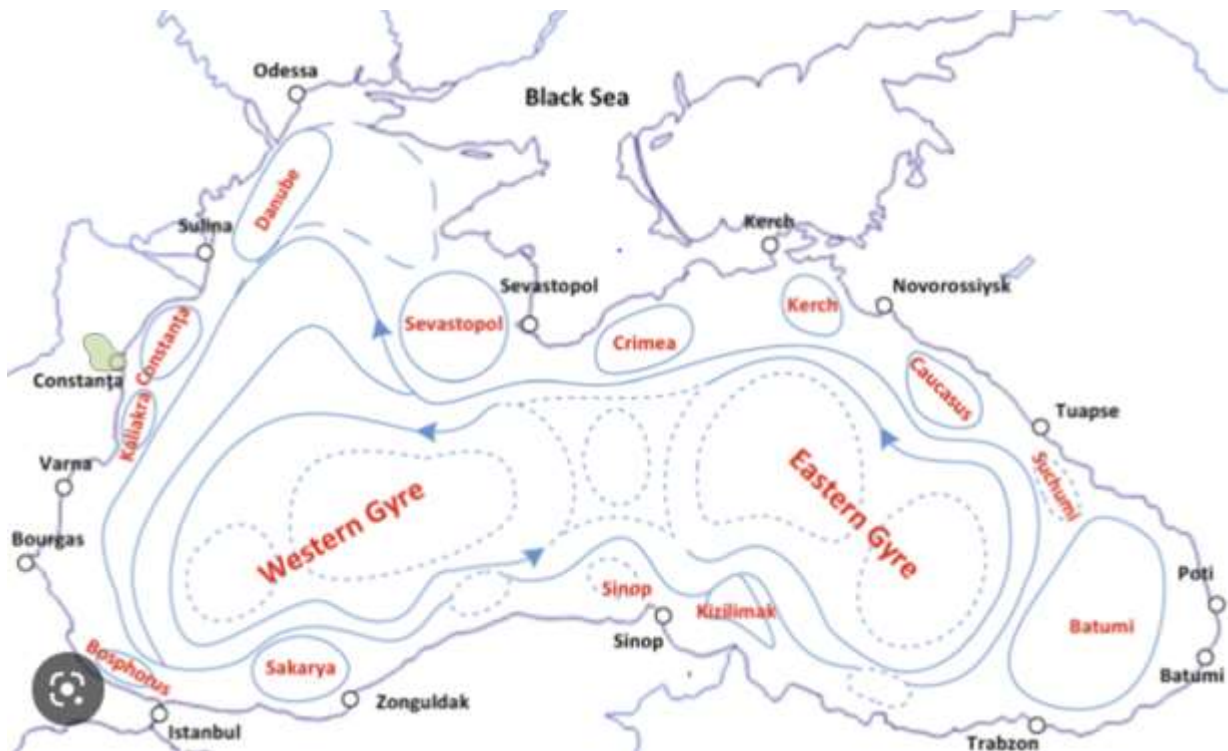
Figure 6-90 – The Rim Current represents a permanent feature of the Black Sea circulating in the Basin following an anticlockwise direction. Small eddies form seasonally along the coastline such the Constanta eddy between Constanta and Sulina and Kaliakra eddy between Constanta and Varna. The area of interest is circled in green.
