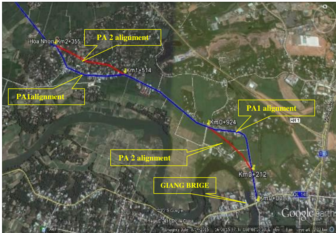
Figure 1-5: Alternative of Alignment section Km0+212 – Km0+924 and section Km+514 – Km2+355
