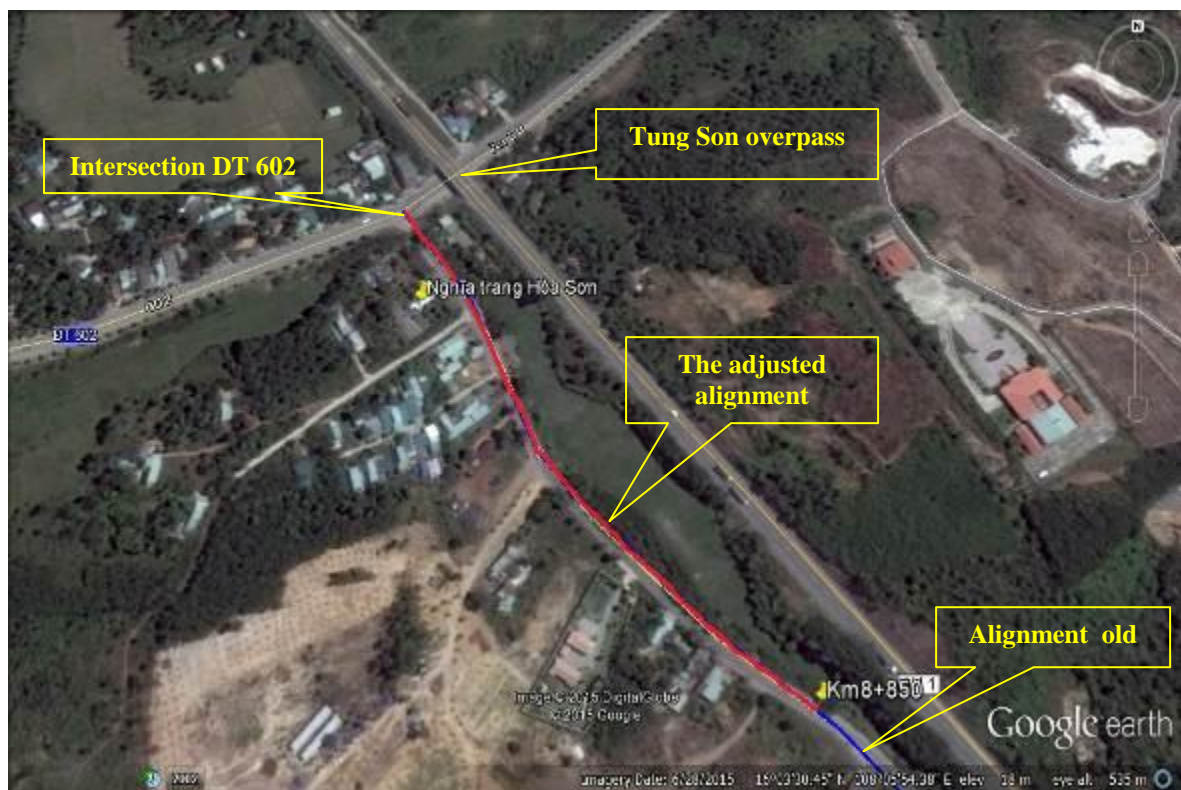
Figure 1-4: Alignment section Km8+850 to the end of route
