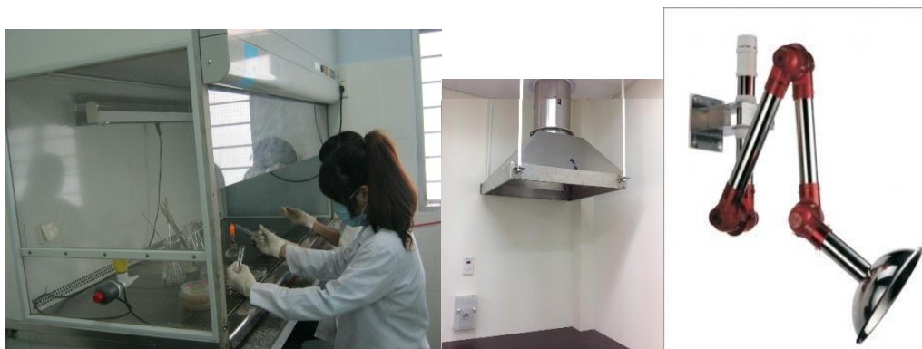
Figure 21. Chemical fume hood, ceiling-mounted fume hood and chemical fume extractor
