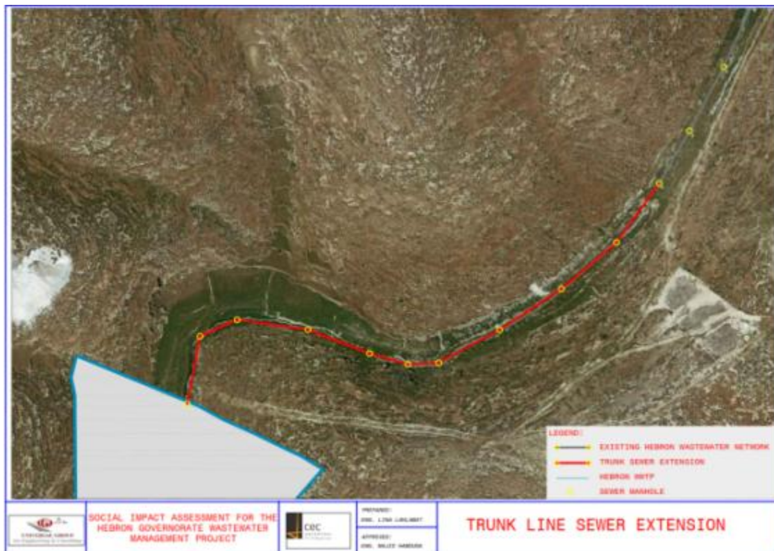
Figure 3.8: Proposed Alignment of Trunk Sewer Extension
