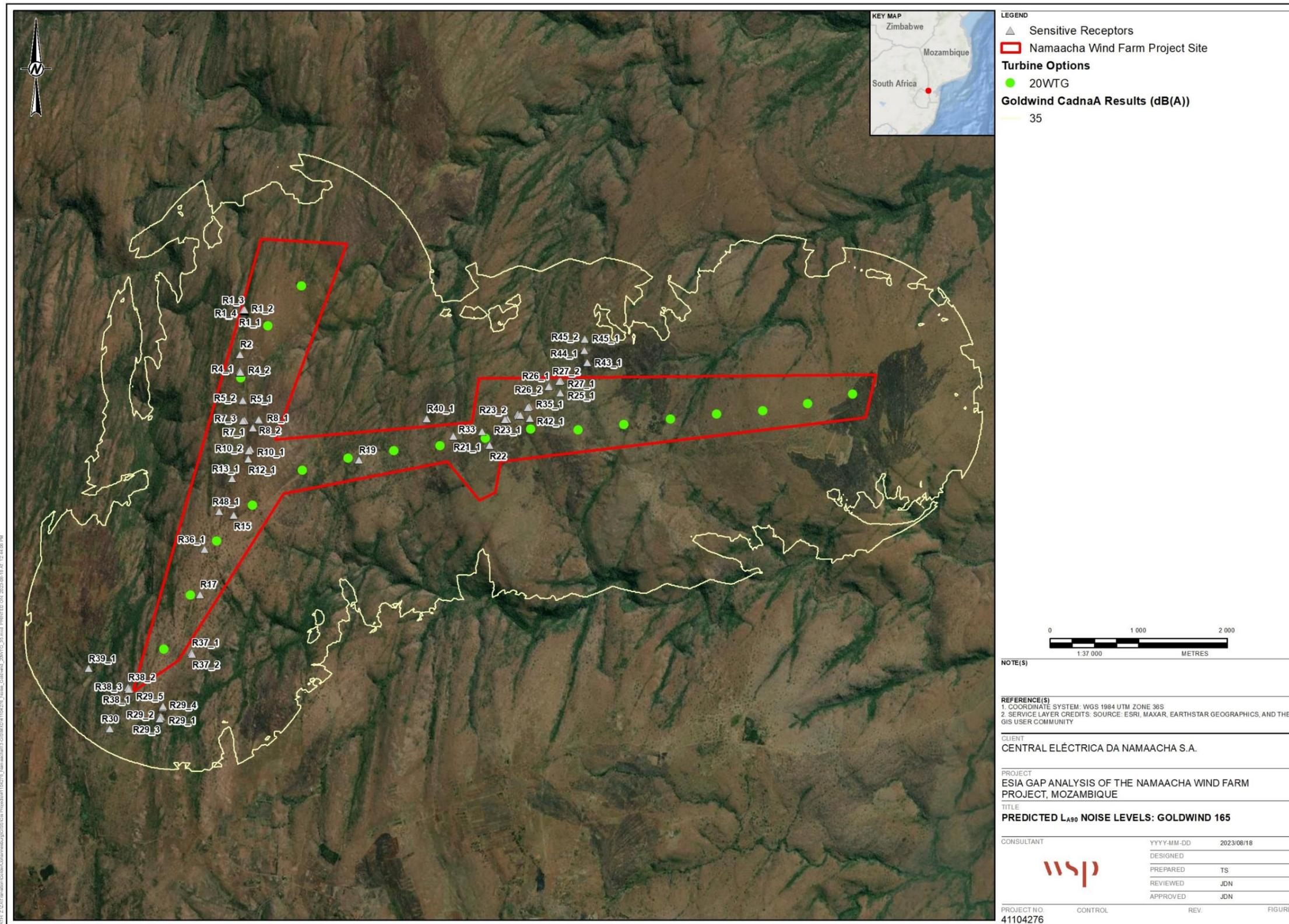
Figure C-3: Goldwind 165 operational design - map depicting the isoline for the predicted ( $L_{A90}$ ) 35 dB(A) level
