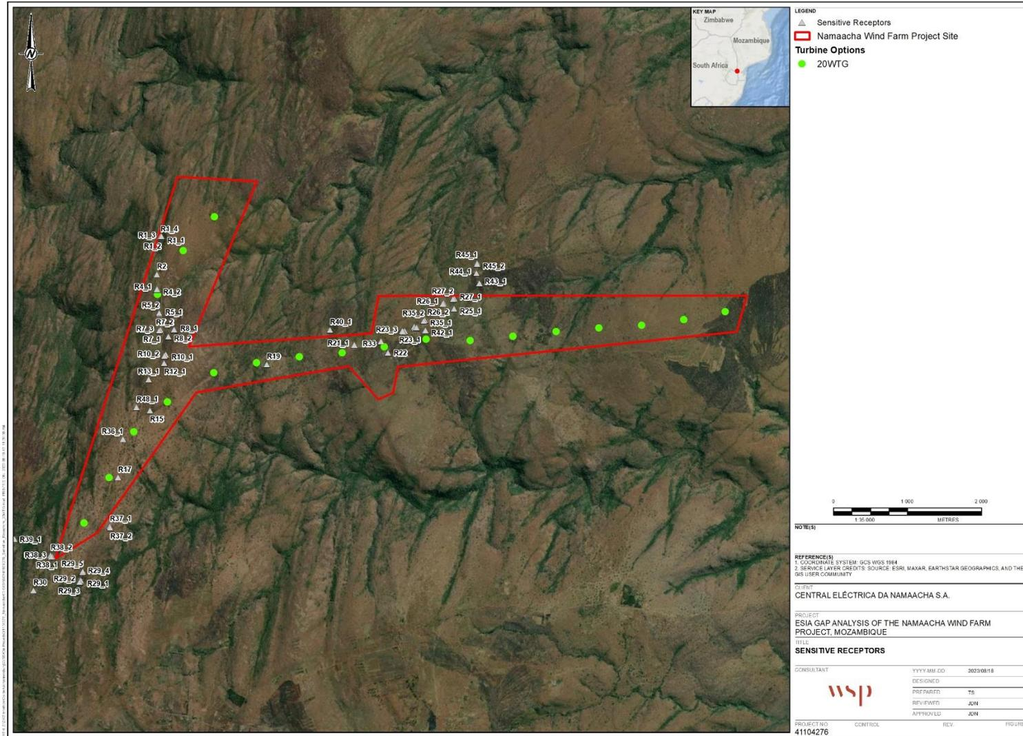
**Figure 4: Receptor map with proposed Goldwind 165 wind turbines layout**
