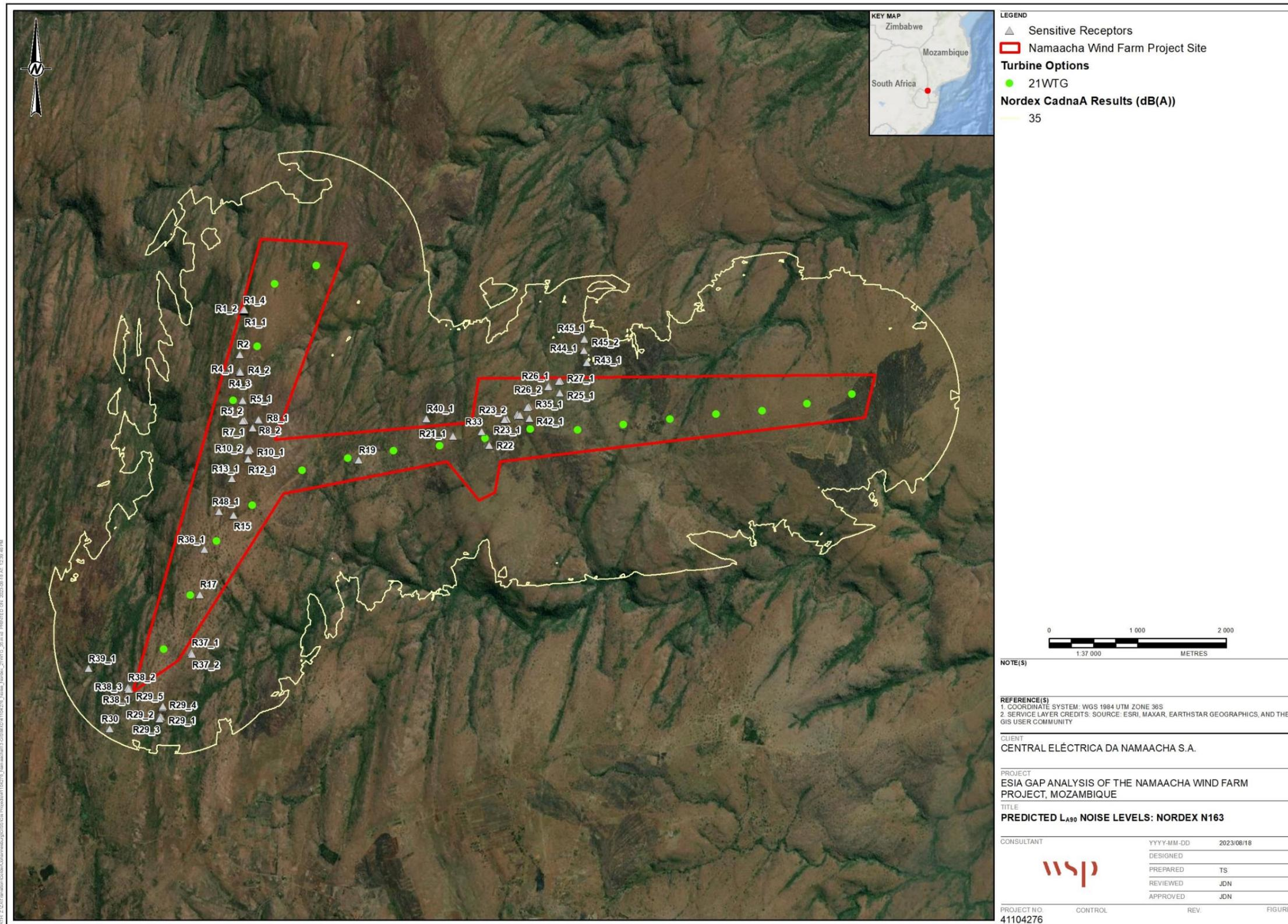
Figure C-1: Nordex N163 operational design - map depicting the isoline for the predicted ( $L_{A90}$ ) 35 dB(A) level
