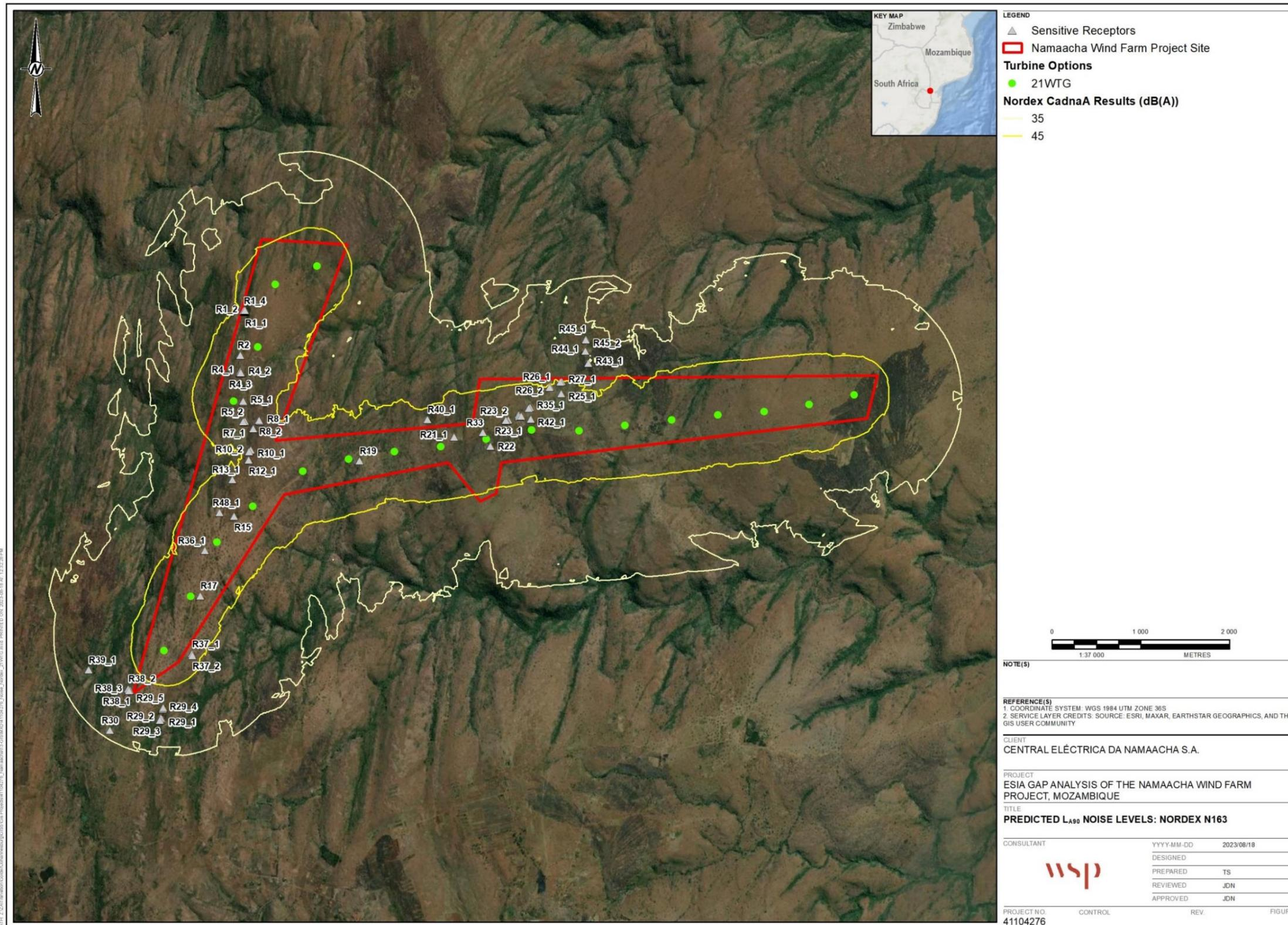
Figure C-2: Nordex N163 operational design - map depicting the isolines for the predicted (L<sub>A90</sub>) 35 dB(A) and 45 dB(A) levels
