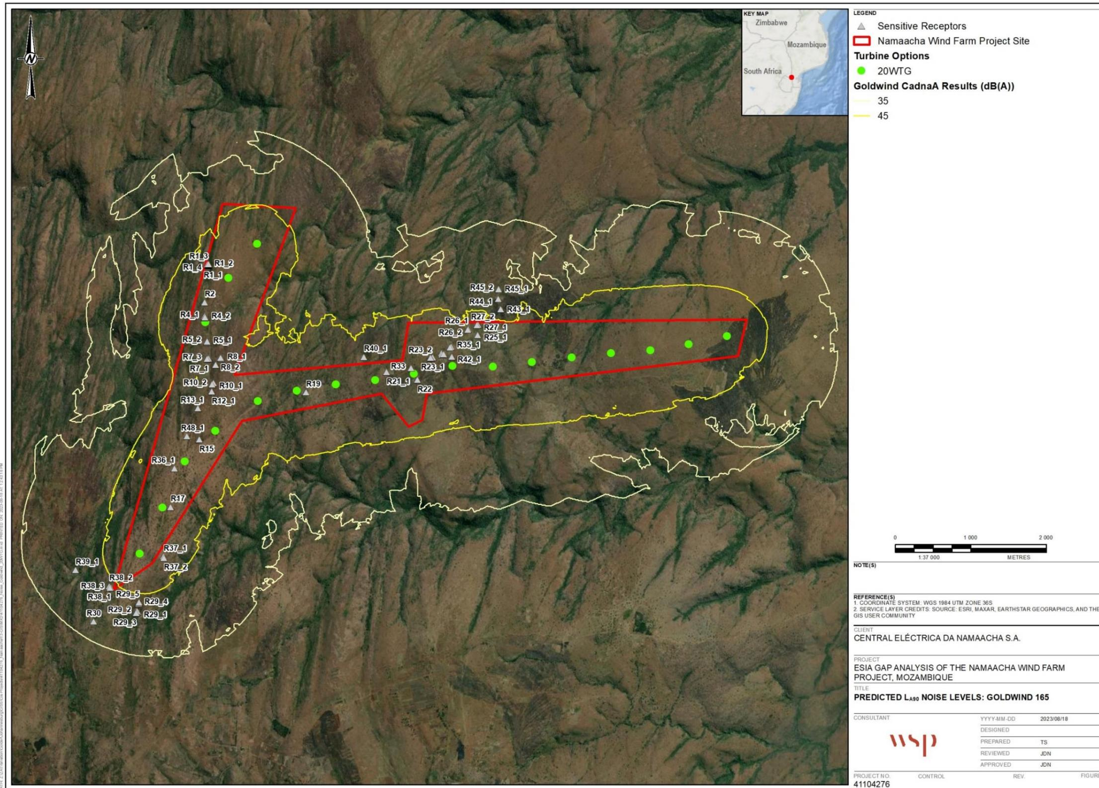
Figure C-4: Goldwind 165 operational design - map depicting the isolines for the predicted (L<sub>A90</sub>) 35 dB(A) and 45 dB(A) levels
