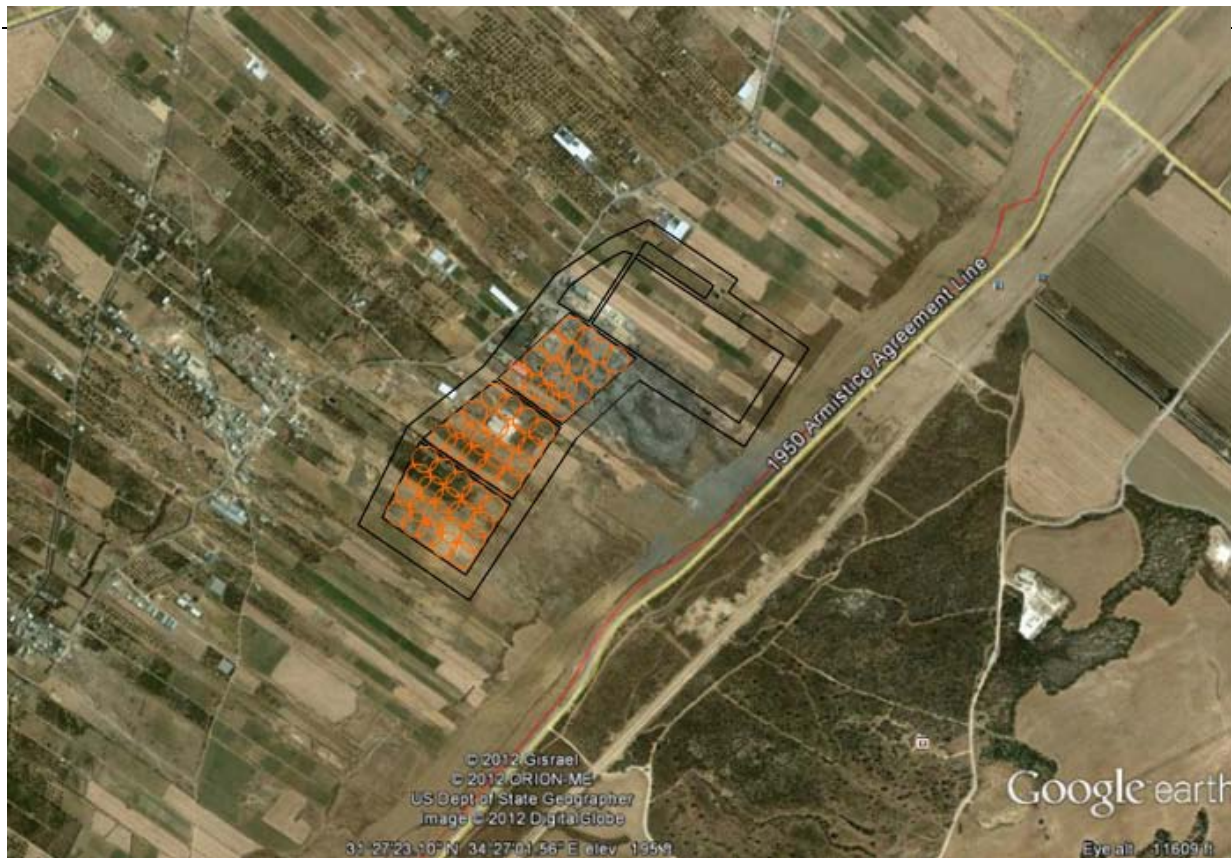
Figure 7A-5: Layout of Johr al Deek landfill – Long term phase covered by 50 gas vents at example locations
