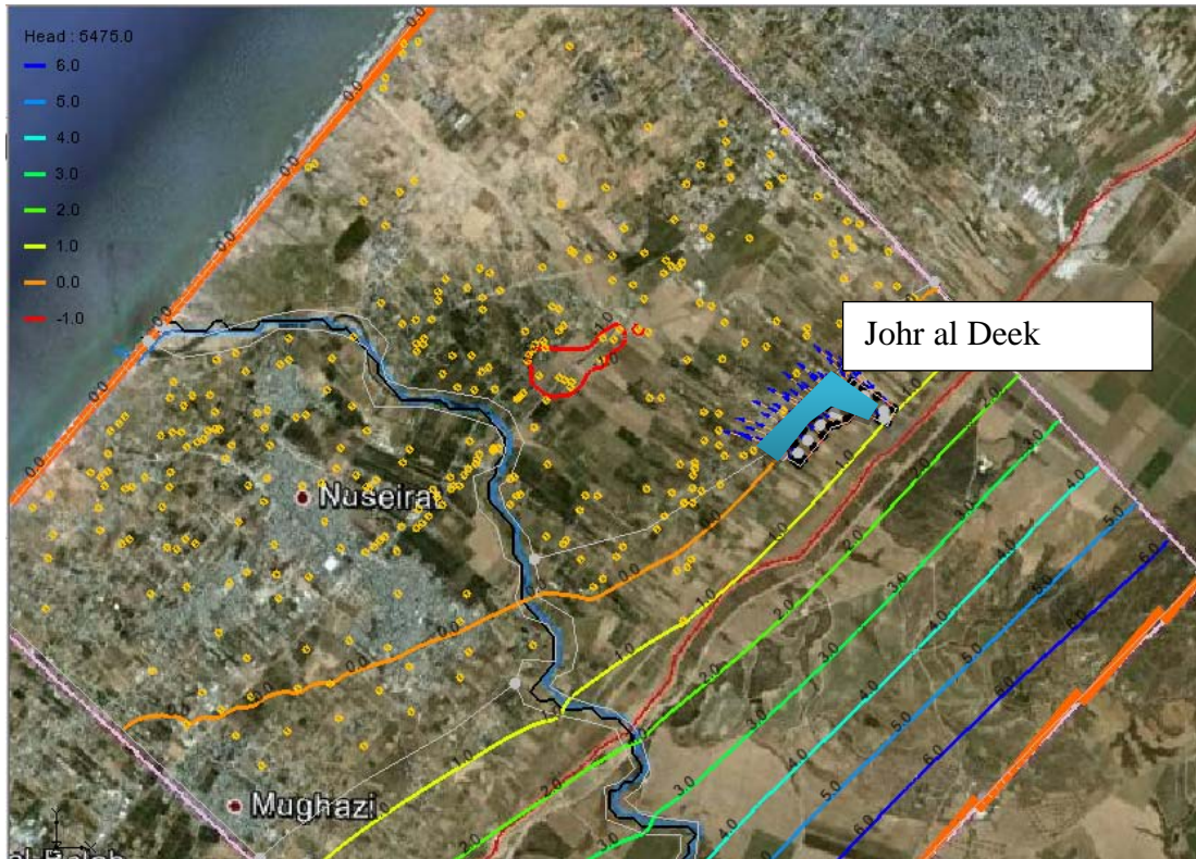
Figure 7A.14 Particles Tracks for Porosity Value of 0.3.
