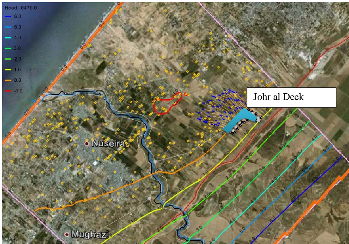
Figure 7A.13 Particle Tracks for Porosity Value of 0.1.
