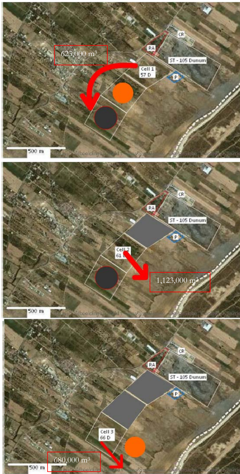
Figure 7A-1: Proposed locations for storing spoil that will be reused in landfill operations
