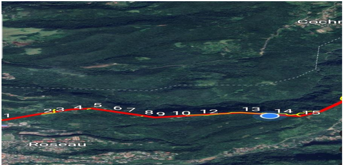
Figure 10: Alignment of the Transmission Line and Pole Locations on the Glasgow Ridge
