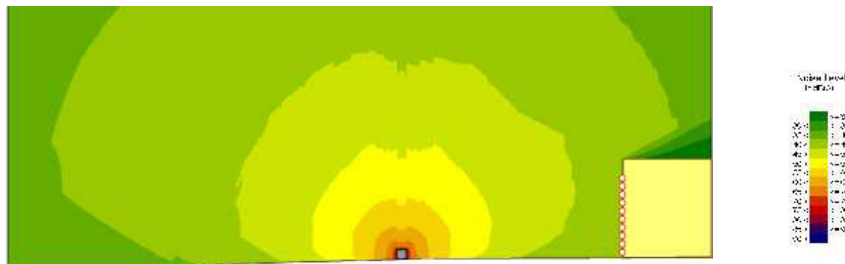
Fig. F.7: Model results for vertical Cross Section BB' – with soundproof enclosure
