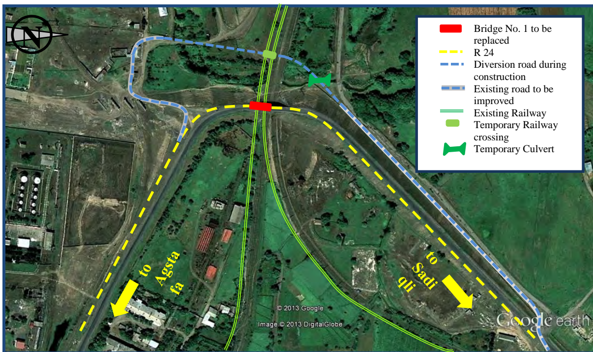
Figure 6: Bridge No. 1 Location Map with Reconstruction Alignment
