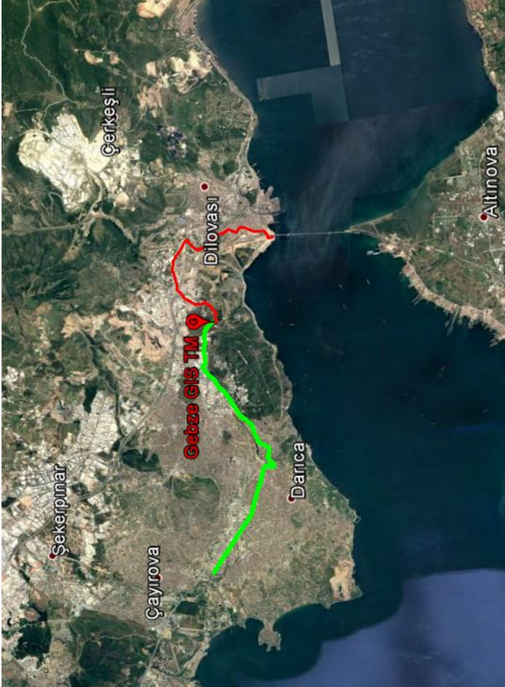
Figure 2 Satellite image depicting UG Cables to connect to Gebze GIS SS-1
