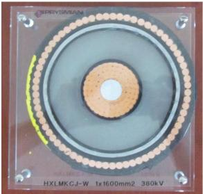
Figure 12: Submarine Energy Transmission Cable
