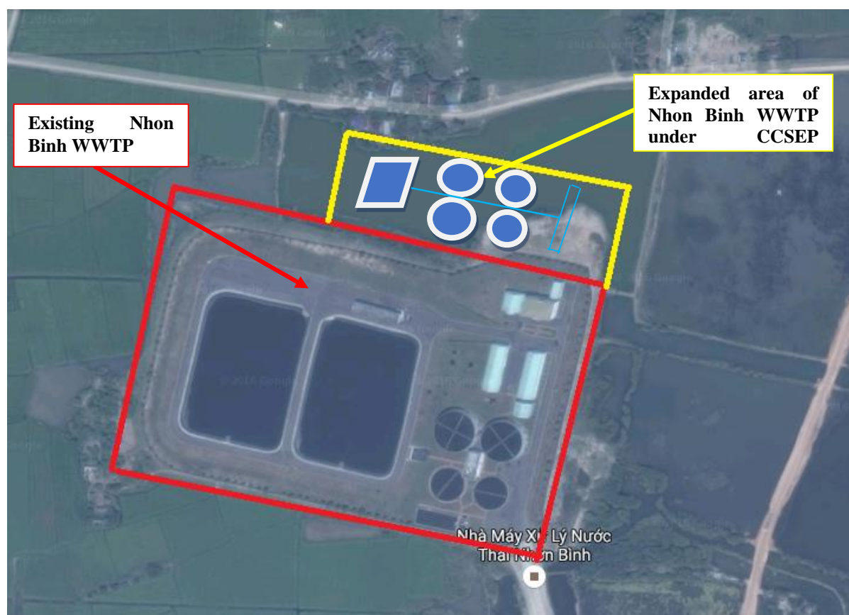
Figure 1.10. The layout of the existing Nhon Binh WWTP and planned expanded area
