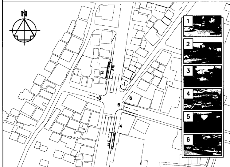
PROPOSED SIGNALISATION OF GOV. M. CUENCO AVE/OLD CARA RD, INCLUDING BRT BUS STOPS AND BUS PRIORITY ON APPROACH TO INTERSECTION
