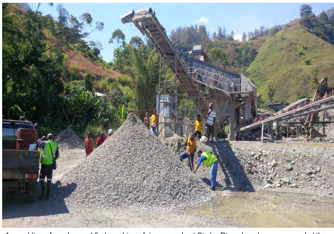
Picture 21: Assembling of the crusher parts inside the airport. Preparing and stabilizing the area for aggregates stockpiling next to the crusher.
