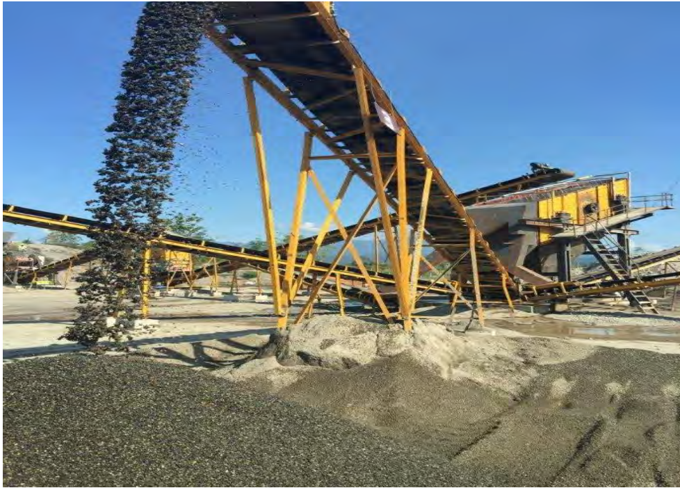
Picture 12: River gravels crushed into aggregates. The gravel is washed when running through the conveyor belt to minimize dust emission.
