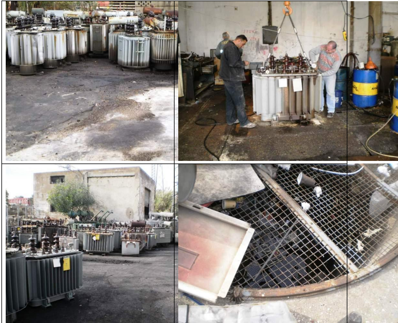
Photograph 5-4: Outdoor storage and repairing of transformers and capacitors at the Baouchriyeh storage site and repair shop leading to PCB leakages on the soil and well (Geoflint 2012)
