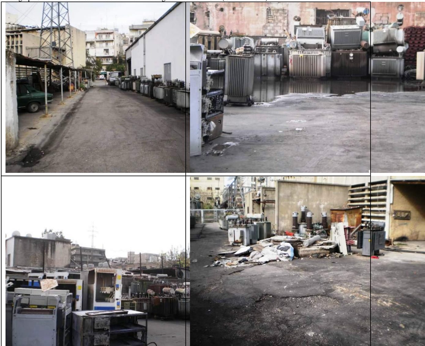
Photograph 5-3: Outdoor storage of transformers and capacitors at the Baouchriyeh storage site and repair shop (Geoflint 2012)
