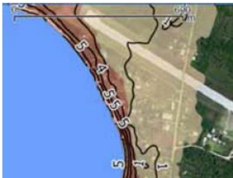
Figure 4.10: Year 2100 flood depths (m) based on an intermediate-high sea-level rise scenario and severe tropical cyclone conditions
