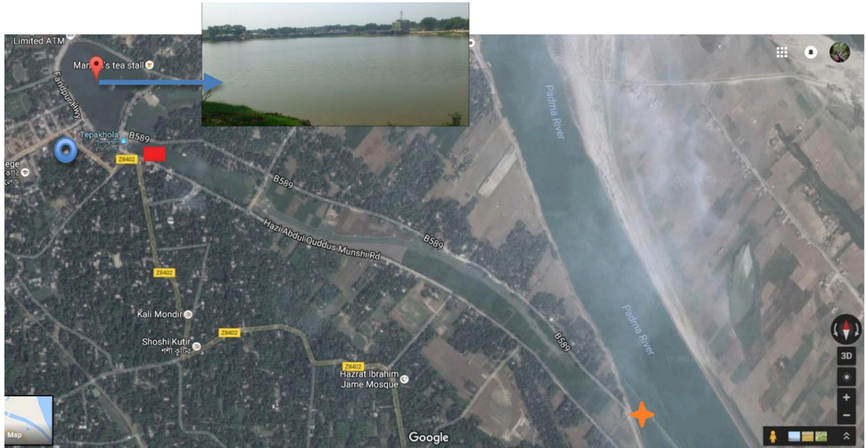
Figure 5: Proposed Intake, alternative intake, impounding reservoir for Faridpur
