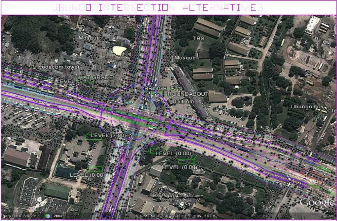
Figure 2.7: Proposed Design Superimposed on the Existing Features (Alternative III).
