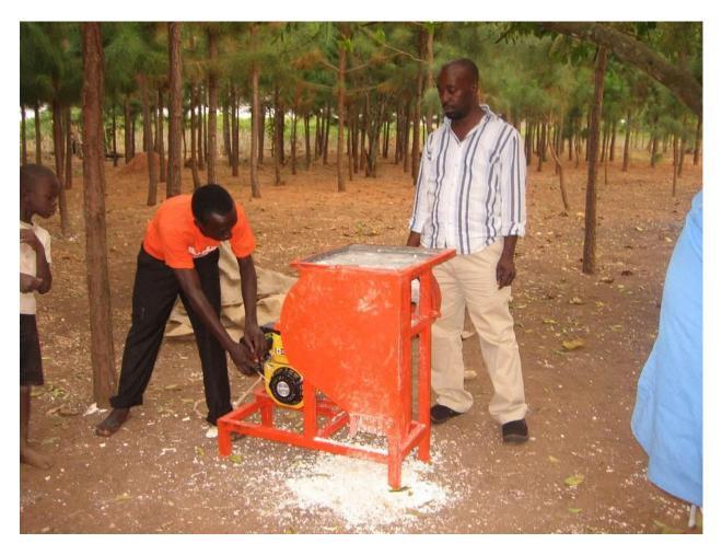
Figure 24: A fabricated machine for slicing cassava right from the garden, the sliced cassava is dried on racks from here
