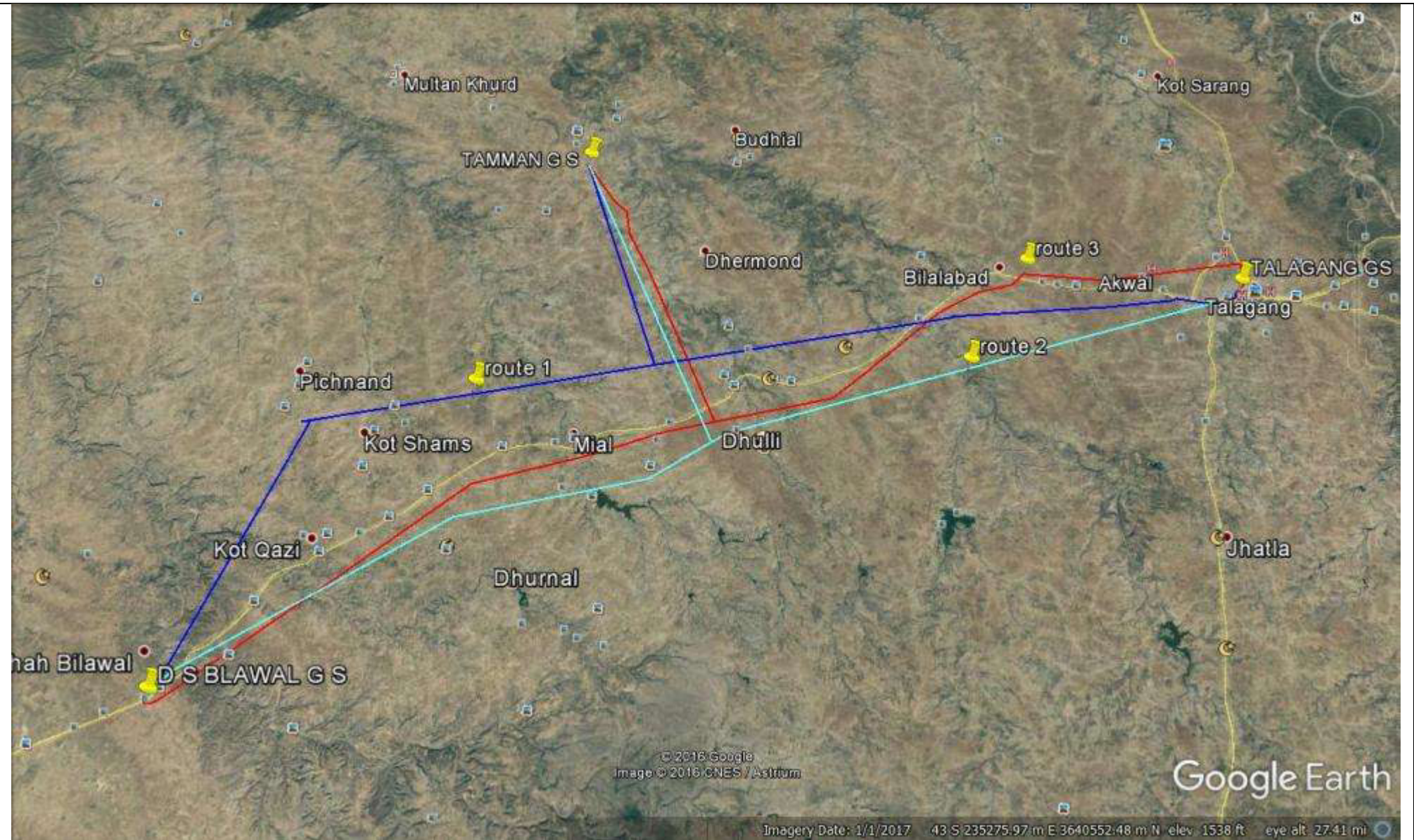
Figure 4.1: Proposed 132 kV Talagang – Danda Shah Bilawal Transmission Line alongwith Alternative Route (Route 3 in red colour is selected as suitable route).
