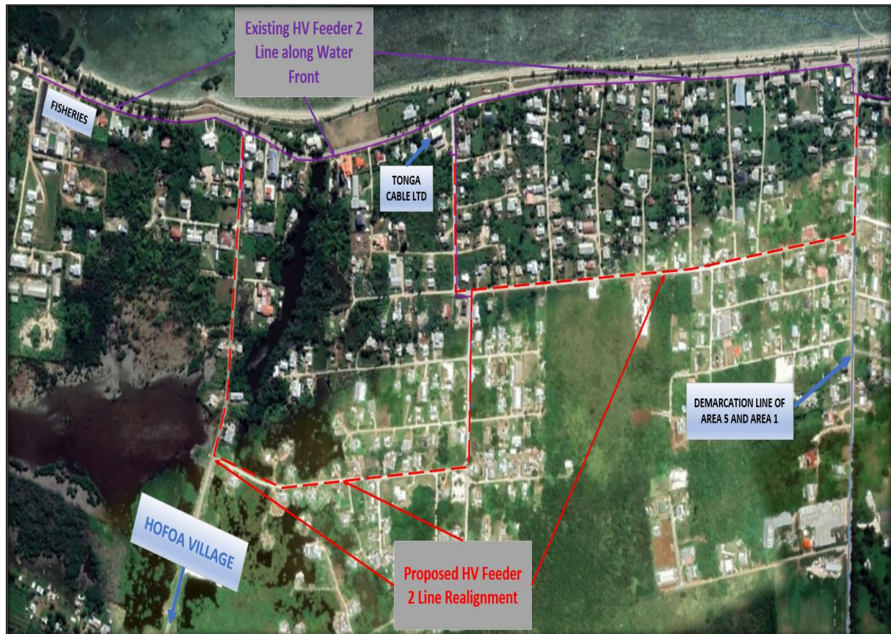
Figure 1: Proposed Realignment of MV and LV for the Waterfront Area
