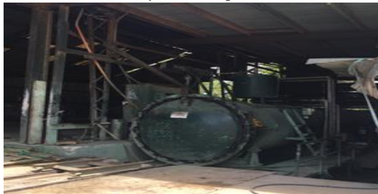
Chemical treatment process using Tanalith C Oxide 670
