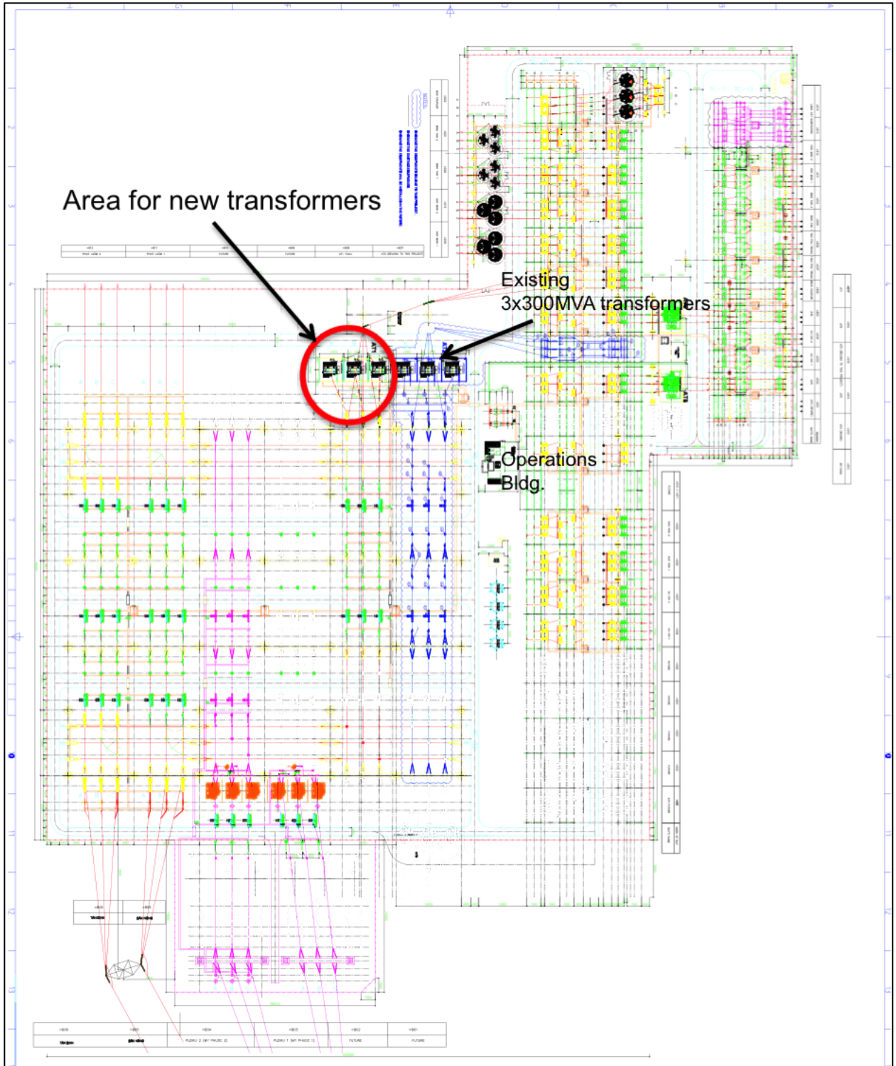
Figure 2: Layout of the 500kV Cau Bong Substation
