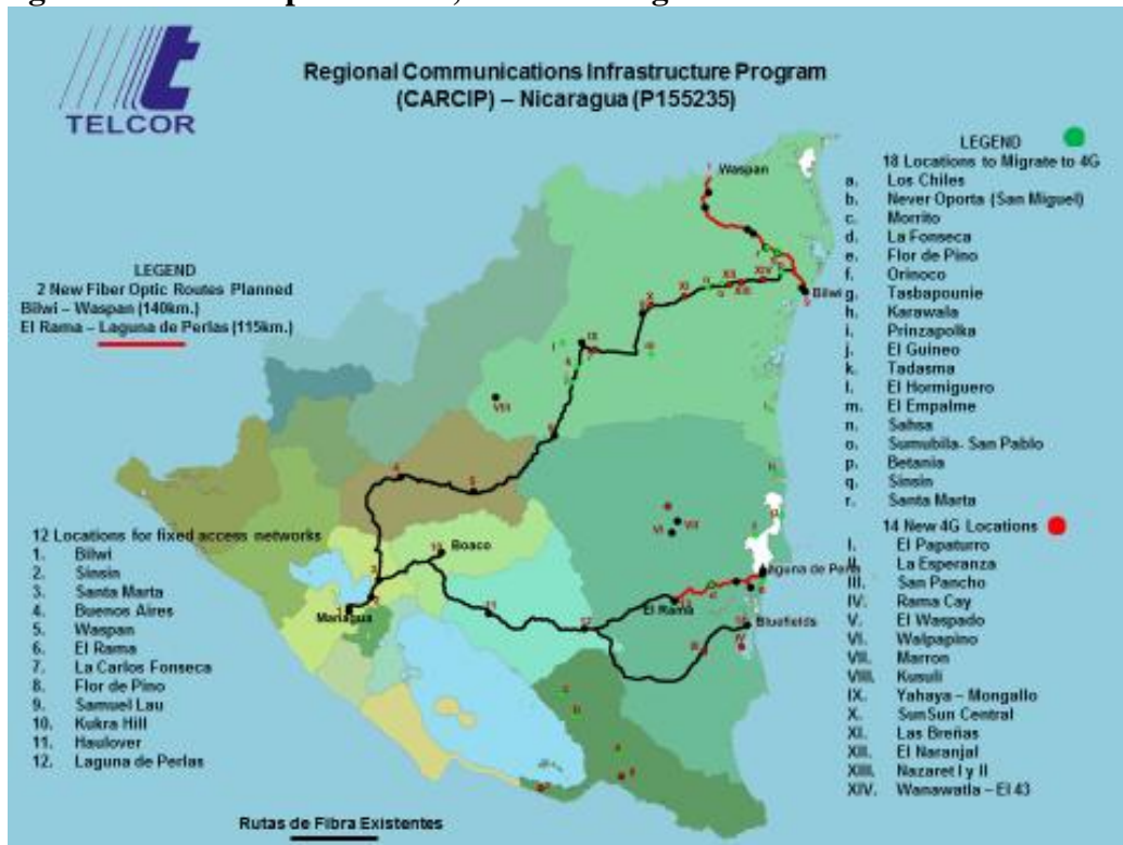
Figure 2.4: Fiber Optic Routes, New and Migrated 4G Towers Under the Project
