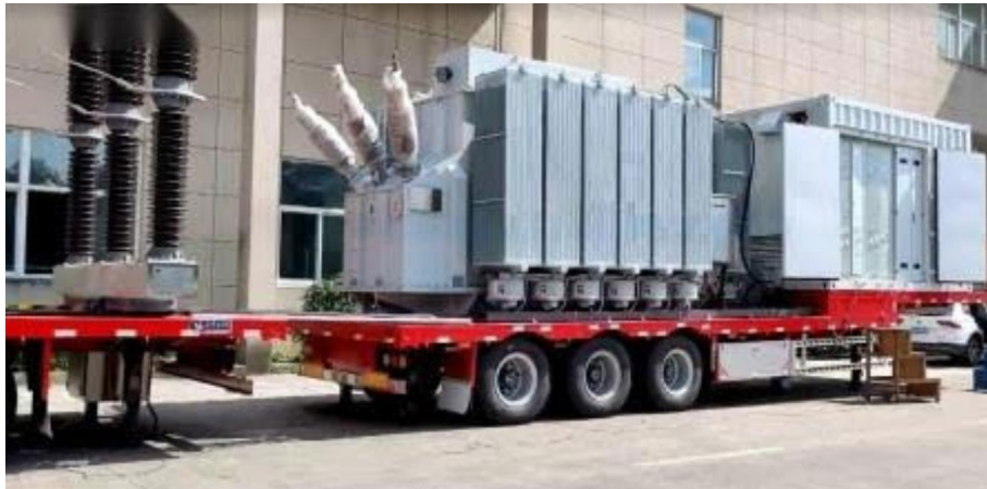
Figure 95: Example of vehicle delivering transformer
