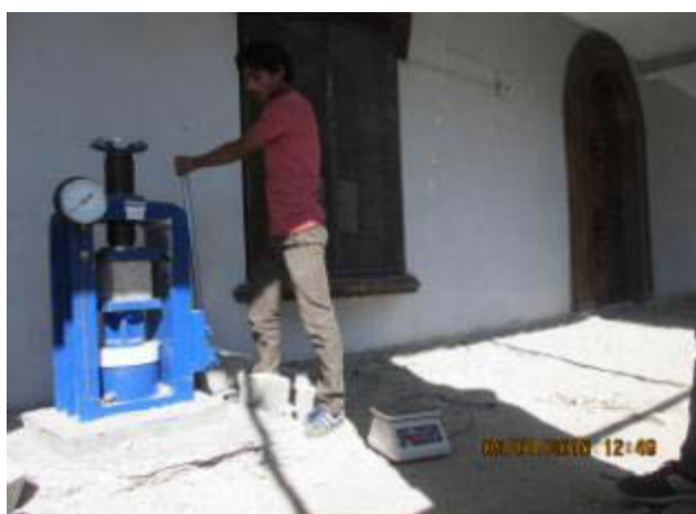
Compressive strength test of concrete cube
