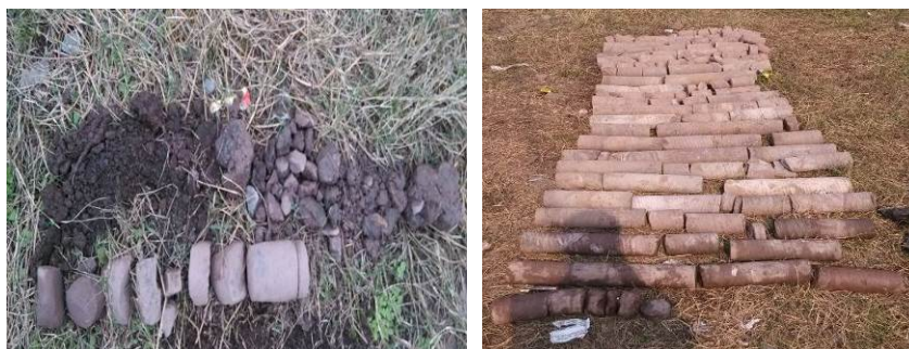
Figure 7 Drilling Record of Ganshui Site: Fill (left) Rock Core (right)
