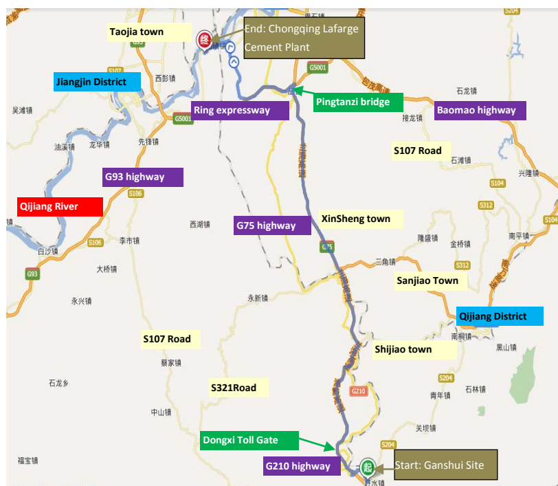
Figure 19 Off-Site Transportation Route of Contaminated Soil
