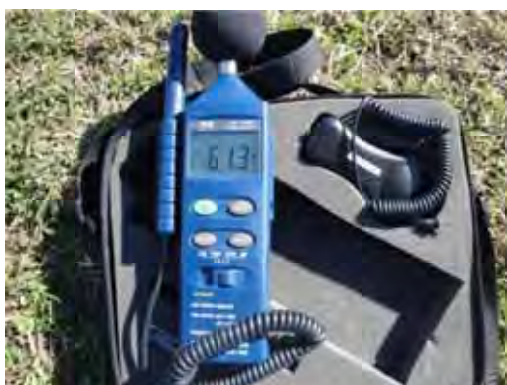
Fig. 4.3. Noise-measuring device PCE-EM882
