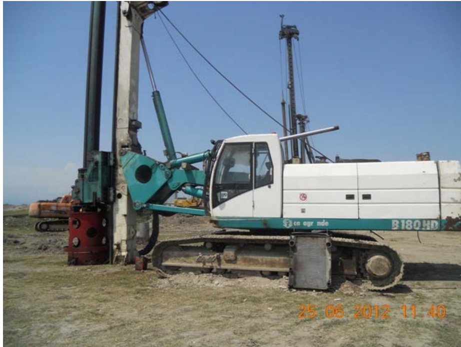
Fig. 3.5 Drilling Equipment Widely Used for Pile Arrangement in Georgia
