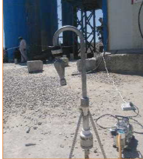
Photos 28 & 29: Air Quality Monitoring at Concrete Batching plants in reporting month (April) on Package 2. (PM 10 & PM 2.5 monitoring at all the three Batching Plants)
