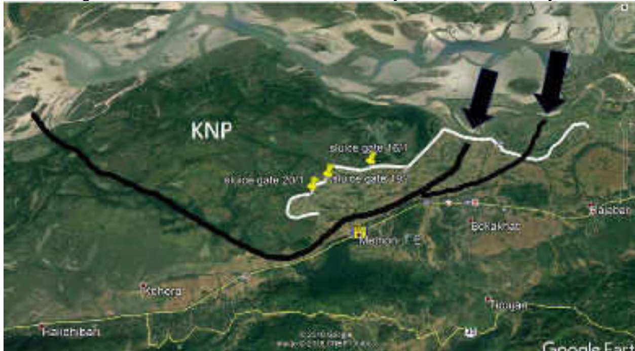
Figure 40: Continuous Attack on the River Bank may Cause Breach on the Dyke
