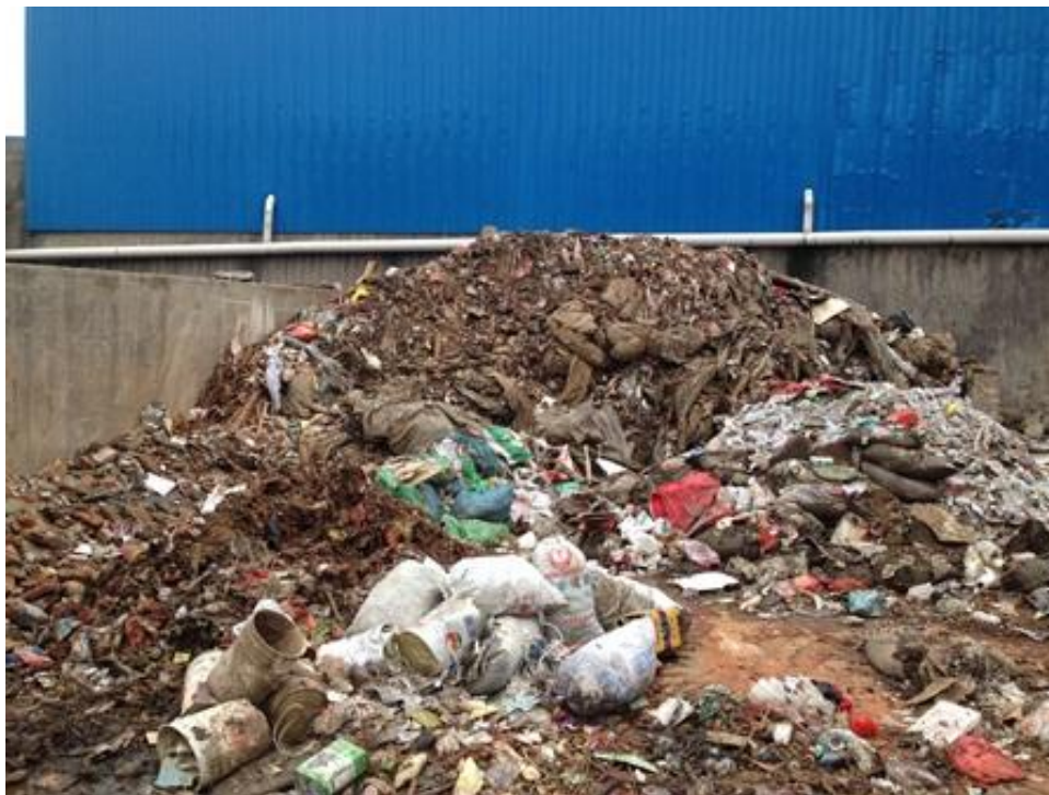
Figure 5-6 Abnormal objects sorted from raw waste in Wuhua incineration plant
